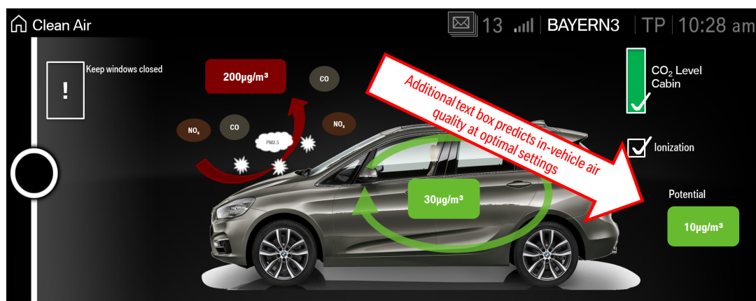
Figure 5.4: Concept of how to signal the predicted best attainable in-vehicle air quality
