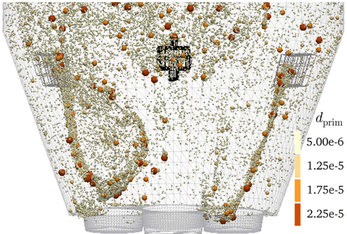
Figure 6.24 Snapshot of the particle cloud approaching the nozzle region after t = 16.2 s. Parcels are magnified by a factor of 2.5. Injection regions are depicted with lines, i.e. water (black) and recirculate (grey).
