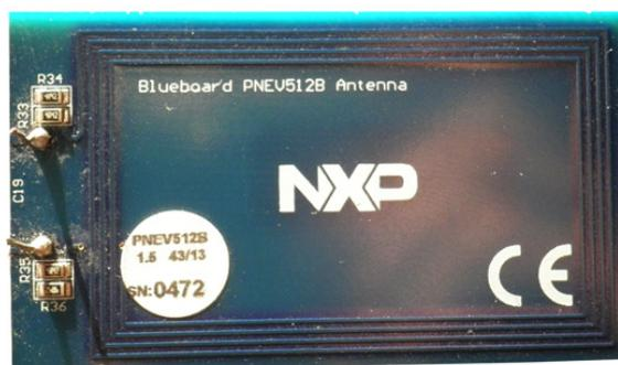
Figure 8.1. – Used sniffer-coil
