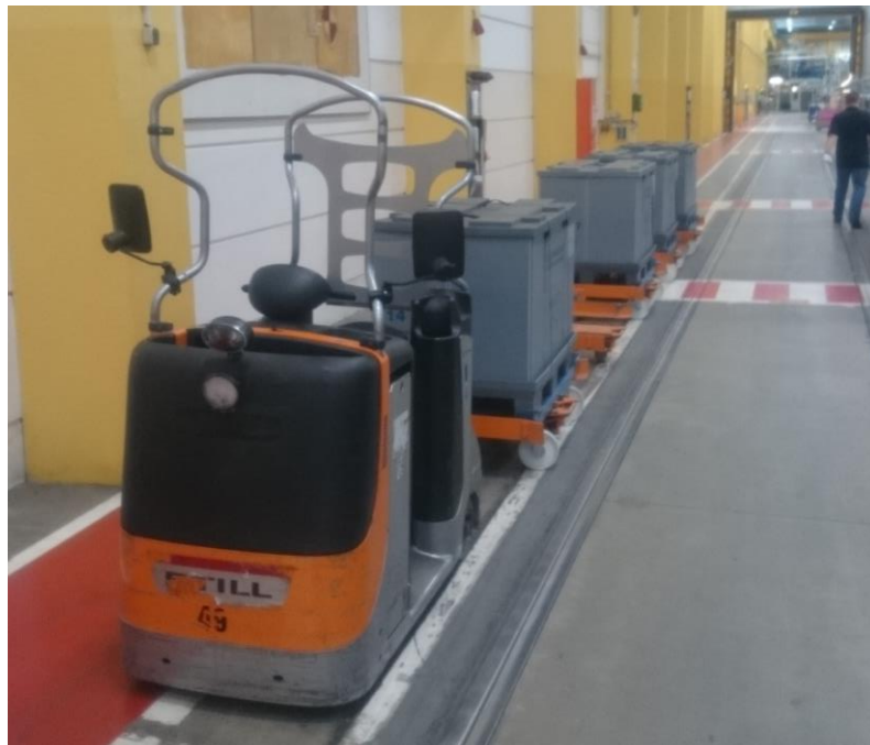
Figure 4-7: Disposal trailer route system
