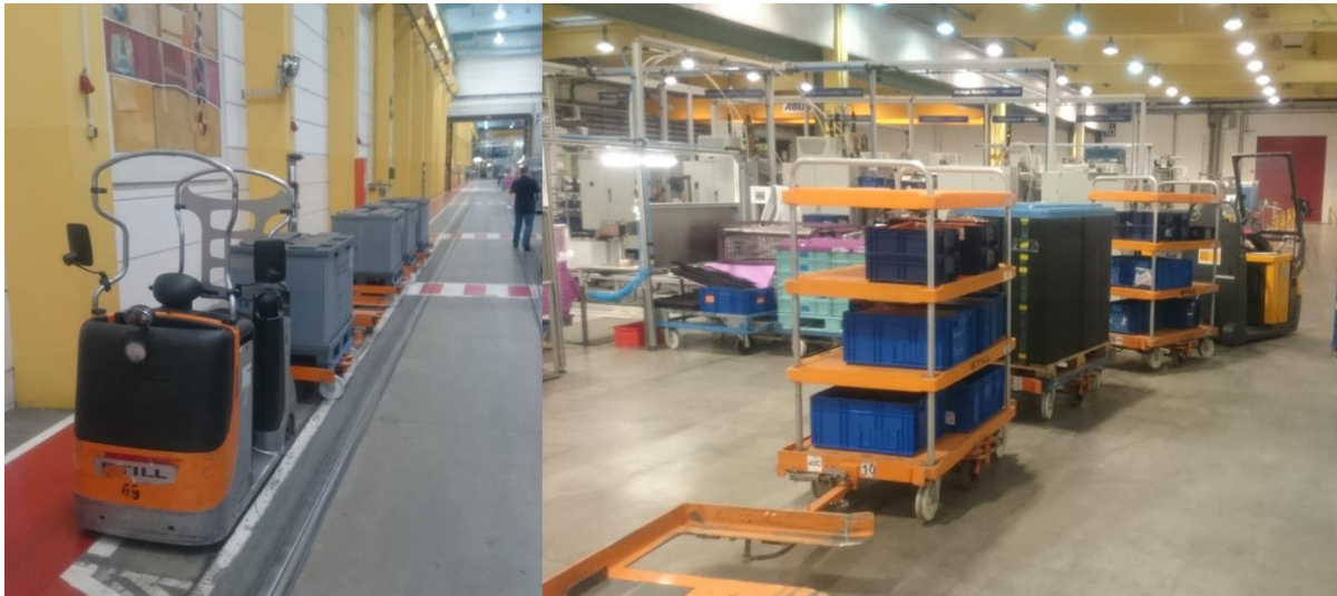
Figure 3-3: Disposal- and supply trailer route system
