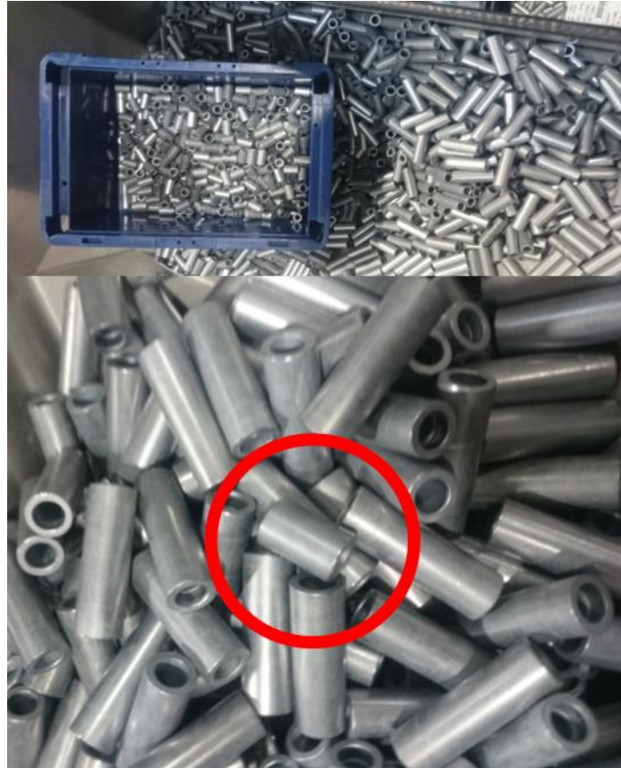
Figure 6-19: Mix-up of supplied materials during the is-measurement
