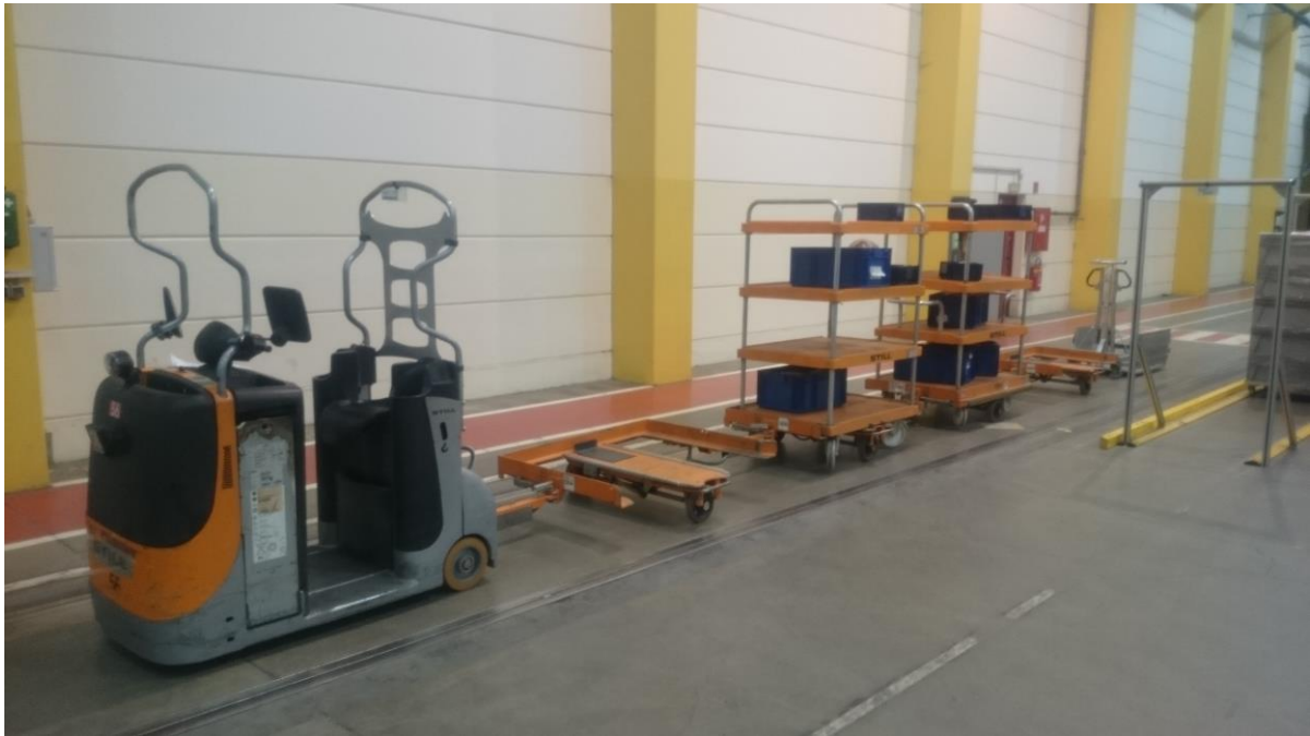
Figure 4-5: Complete assembled supply train
