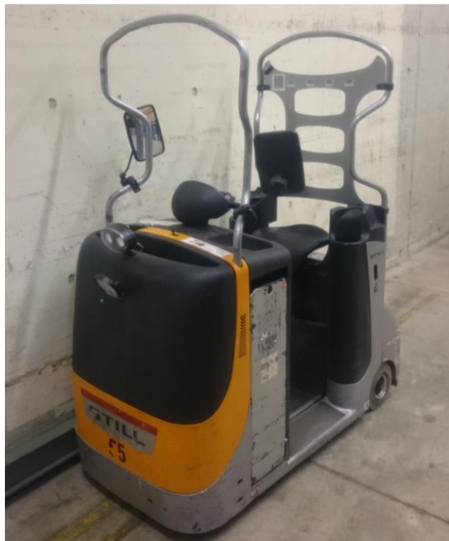
Figure 4-2: Tractor unit of a trailer route system
