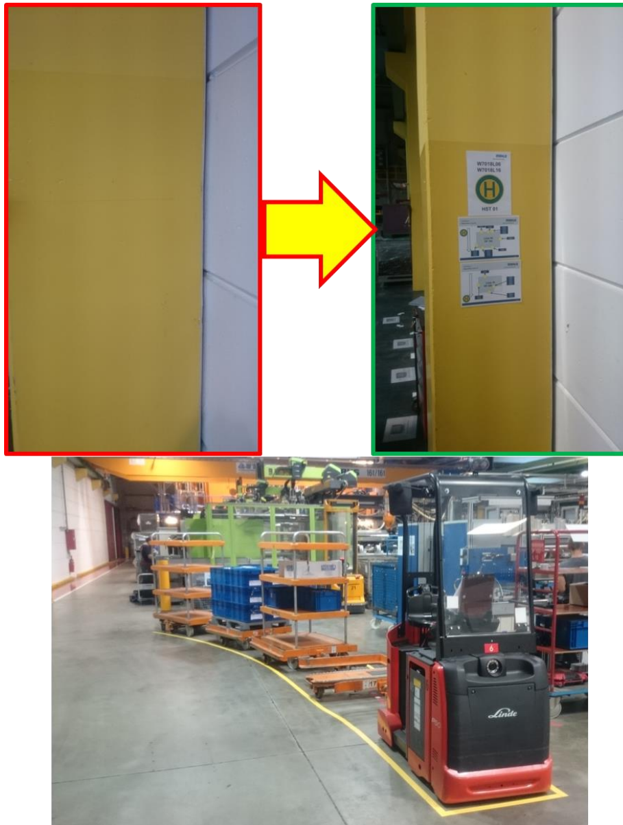
Figure 7-4: Line layout signs and stopping station
