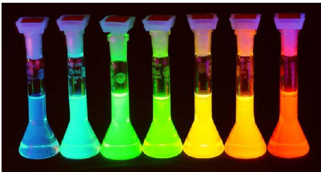
Figure 3. CdSe quantum dots with different particle sizes (13)
