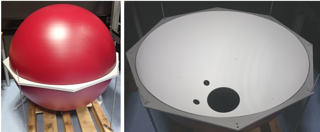
(a) Integrating sphere before assembly onto the rack.
