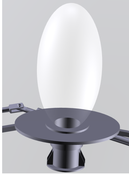
Figure 3.4.: Illustration of the lamp baffle around the socket.
