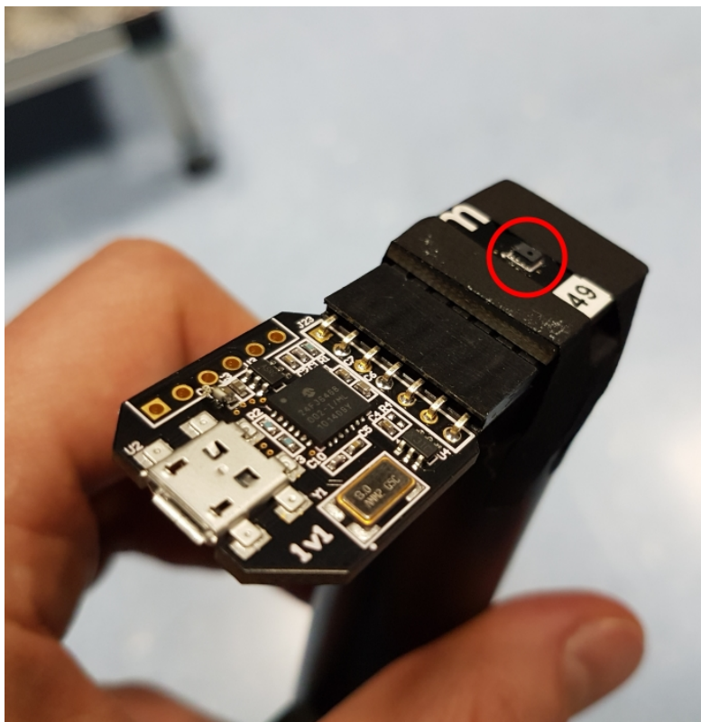
Figure 4.1.: Sensor fixed on the mounting. The red circle highlights the sensor.
