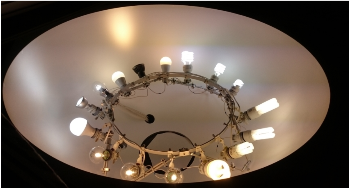
Figure 3.8.: Lamp-frame with lamps, before the lamp baffles were attached.
