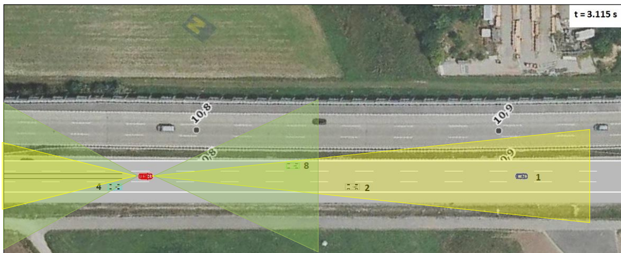
Figure 3-32: “AHDAS” Simulation: Ego-car has the same velocity than the car ahead and decides to start a lane change to the left side
