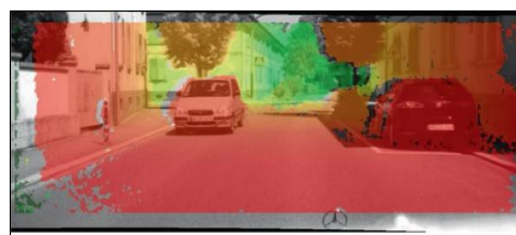
(b) visualisation of distance information. Red areas are closer (< 10m), green areas are distant (> 60m)
