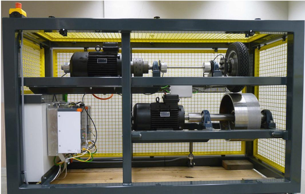
Figure 5.1: Test bench for investigating the power-train control concepts.
