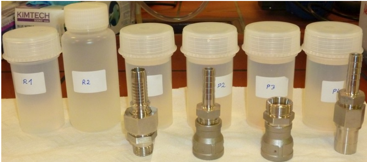
Figure 41: Austenitic stainless steel samples and filled bottles after corrosion test - Overview (Test protocol: DI water, 3 days, 90 °C)
