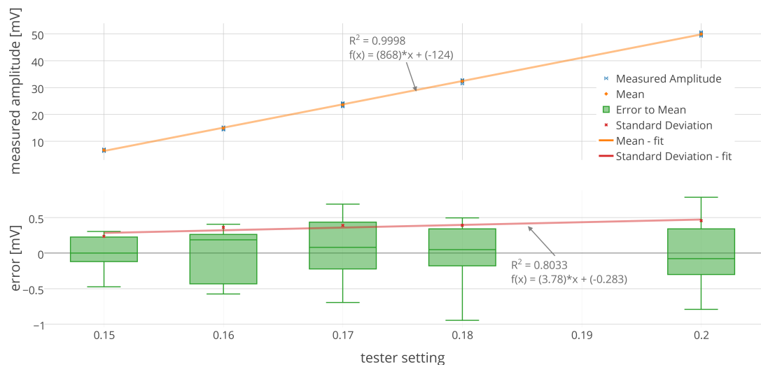
Figure 6.7: Measured data, mean value; error in regards to the mean value and the standard deviation are displayed. The tester settings are not calibrated; the results increase linearly with the input. Amplitudes below 10 mV show errors inside the \pm 2\% limits.
