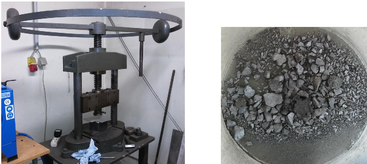
Figure 4.20: (a) Press at the IWS and (b) nugget after pressing
