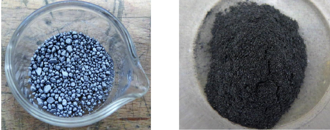
Figure 3.8: (a) Chromium, as purchased and (b) chromium, after milling.
