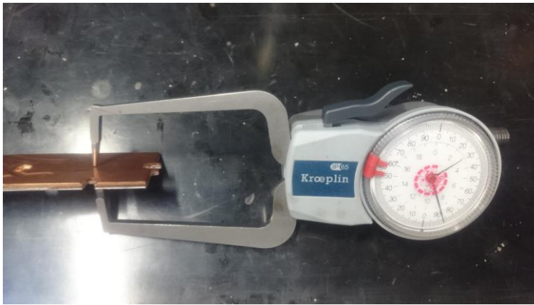
Figure 5.5: Measuring procedure with a standard thickness gauge (Michael Riesenhuber 2016)
