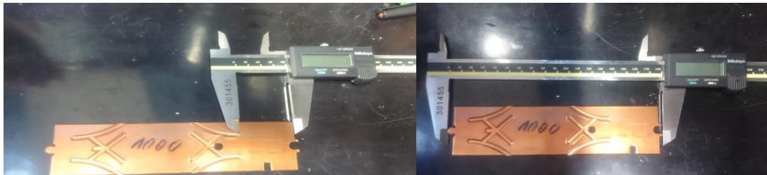
Figure 5.4: Length measurement procedure of plate (Michael Riesenhuber 2016)
