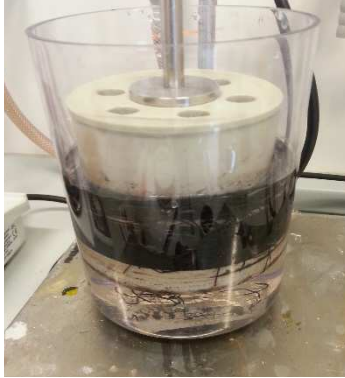
c) Washing of \text{CuS} coated fibers
