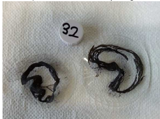
f) \text{SnS} containing fibers after drying
