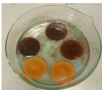
a) Cellulose films during regeneration
