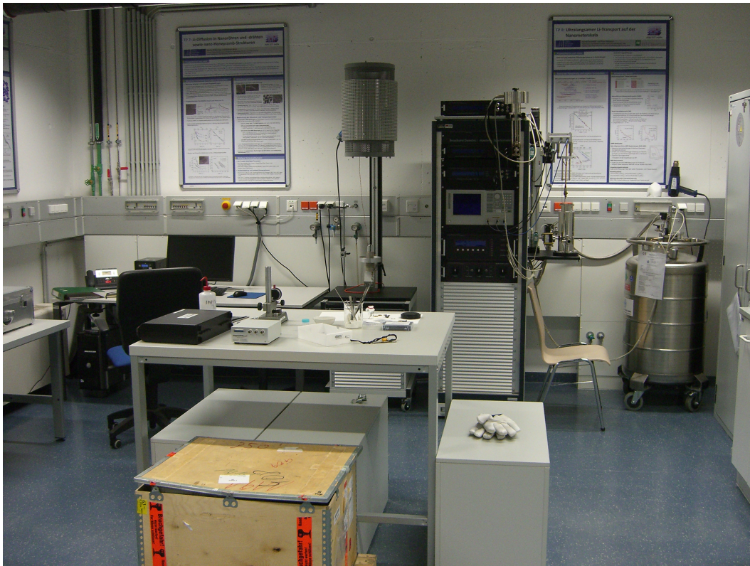
Figure A.3: Photograph of the impedance spectroscopy workstation Concept 80 (Novocontrol).
