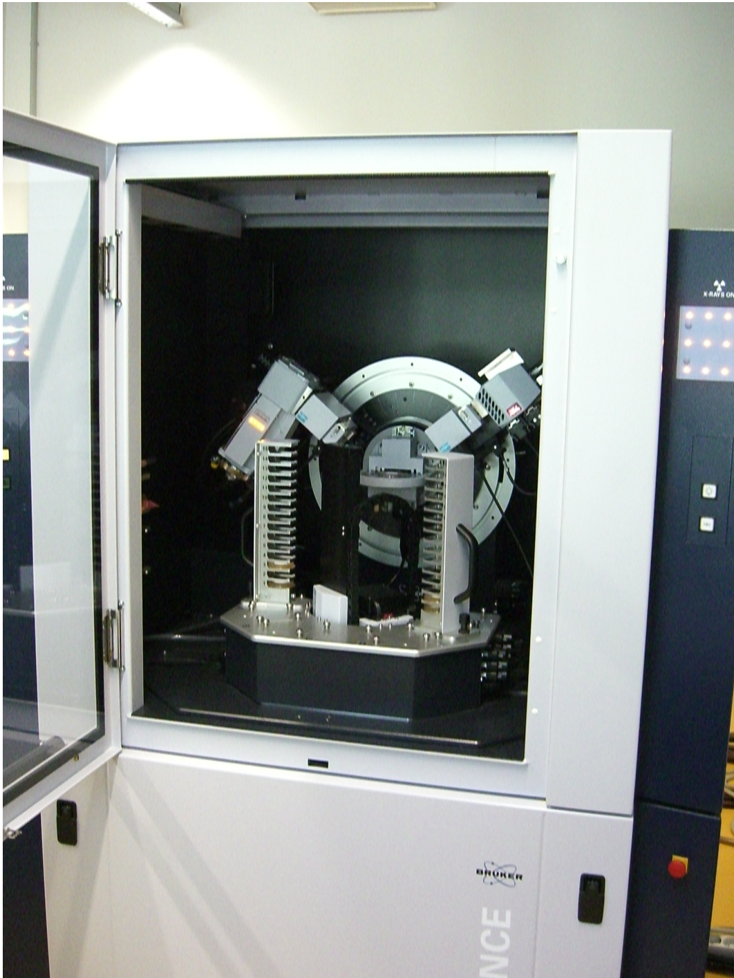
Figure A.1: Bruker D8 Advance diffractometer with Bragg Brentano geometry.
