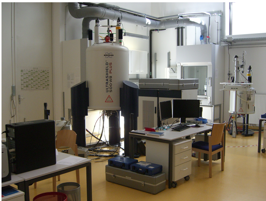
Figure A.2: Photograph of the solid-state NMR spectrometer workstation Bruker Avance III 500.
