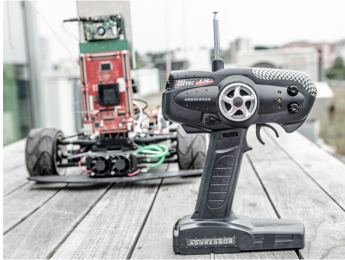
Figure 3.9: RF remote for the scaled vehicle.
