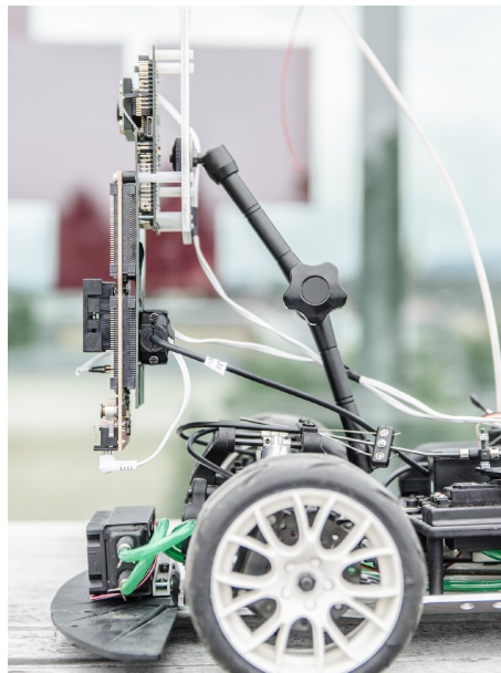
Figure 4.5: Flexible arm on the scaled vehicle.
