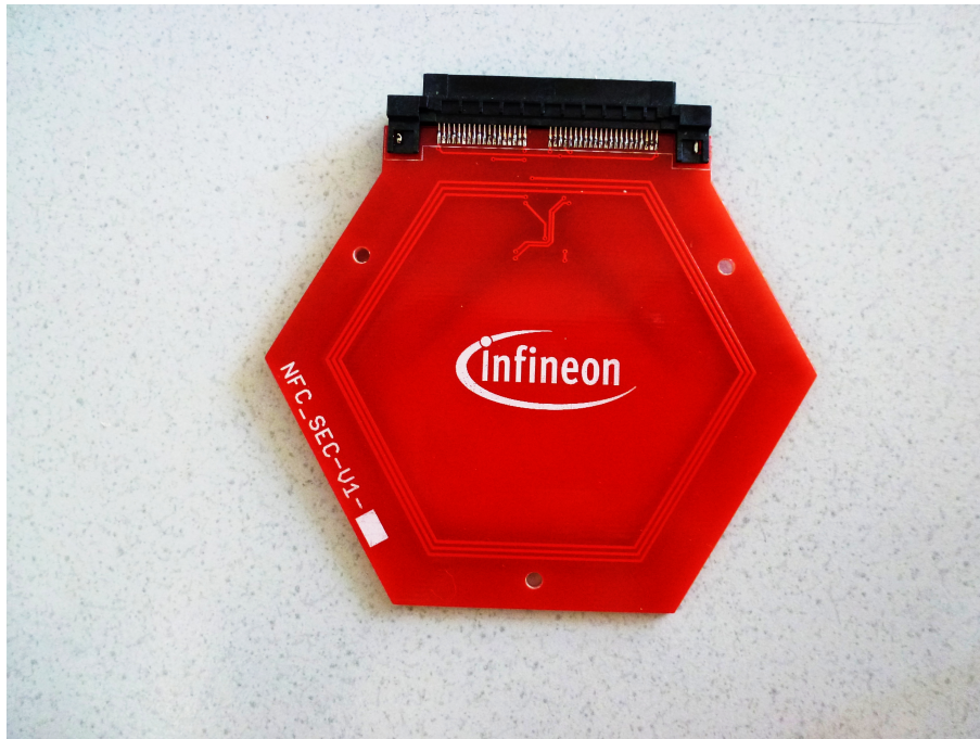
Figure 4.4: The CUTIN hardware prototype comprises a host controller, security controller and an NFC antenna on an Infineon evaluation board.
