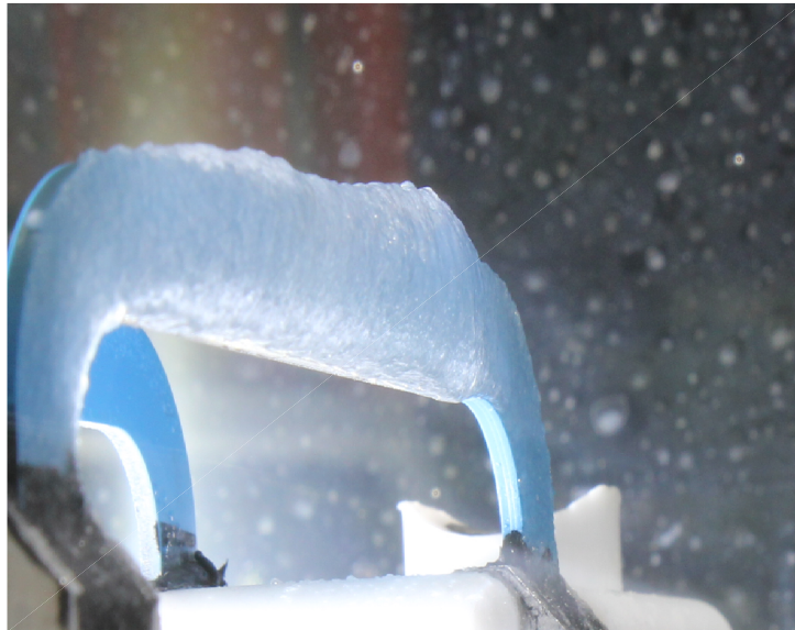
Figure 2.22: Picture of the ice layer on the sensor right before the heating cycle.
