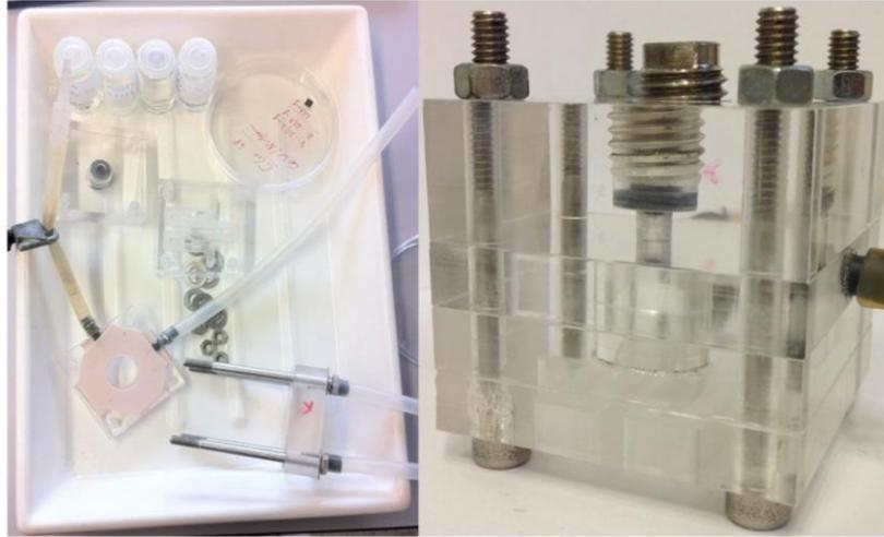
Figure 10: In-house made hydrogen release cell; spare parts (left) and assembled cell (right).
