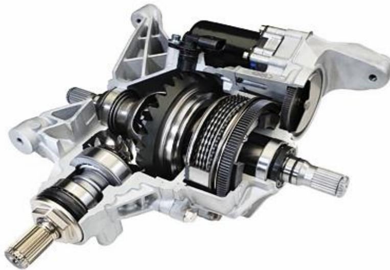
Abbildung 7.2: GKN Sideshaft Disconnectsystem [14]
