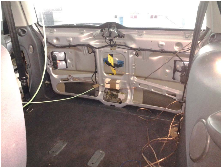
Figure 87: Antenna position - trunk middle
