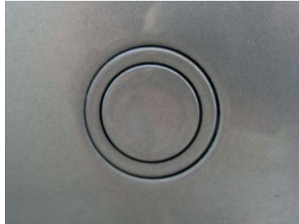
Figure 6: Audi A4 ultrasonic sensor [10]
