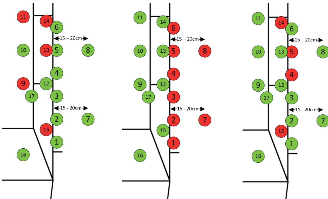
Figure 119: Setup 3 with fixed alarm boundaries and 2dB, 1GHz for: no false alarms (17 cm), no misses (79 cm), min. wrong decision (28 cm)
