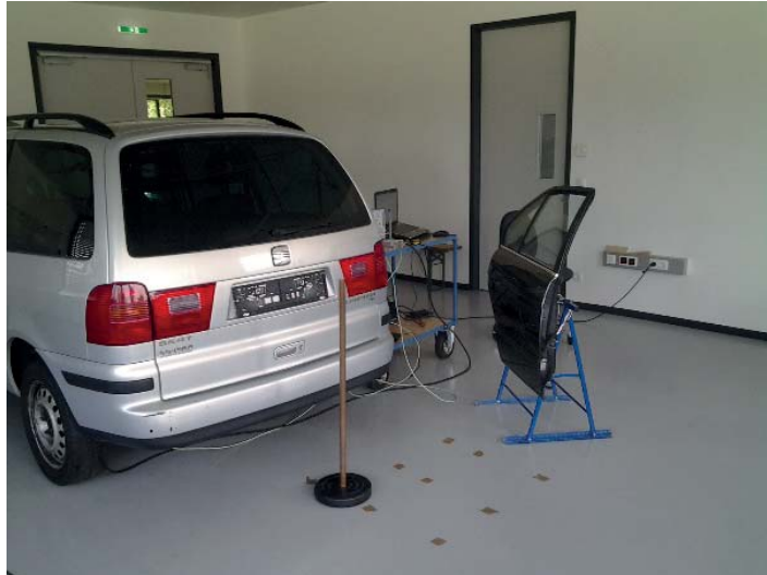
Figure 66: Setup with 45° inclined car door at 50 cm distance
