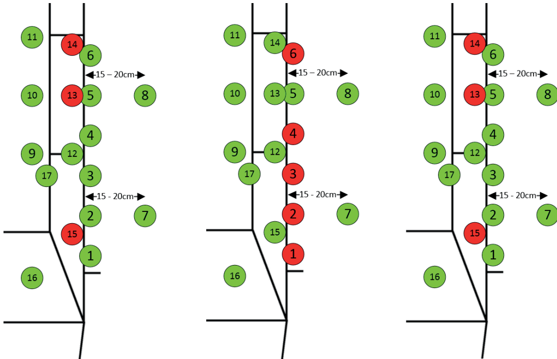
Figure 118: Setup 3 with fixed alarm boundaries and 1dB, 1GHz for: no false alarms (17 cm), no misses (79 cm), min. wrong decision (28 cm)
