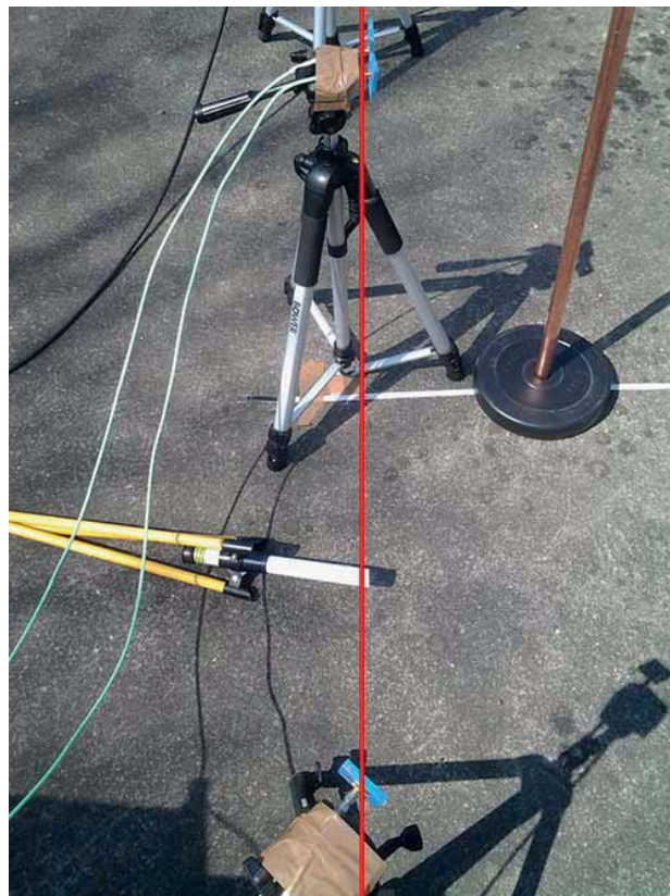
Figure 8: photo of 45° rotation of side antennas
