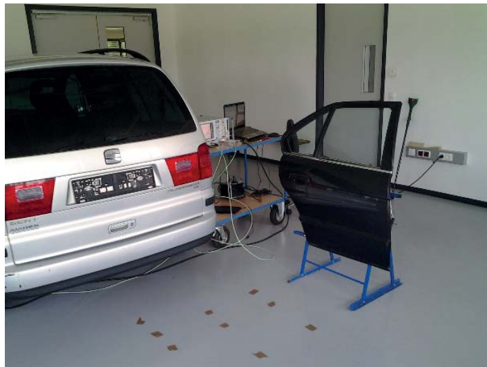
Figure 65: Setup with parallel car door at 30 - 40 cm distance
