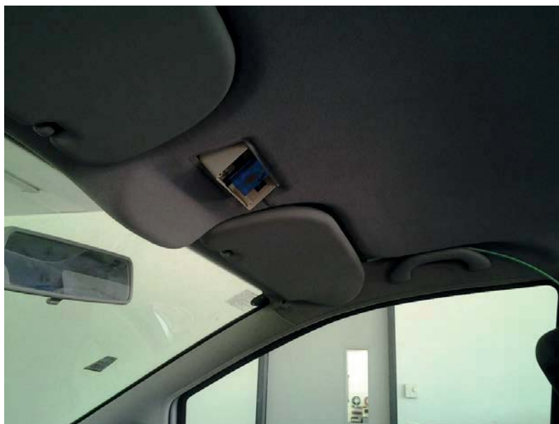
Figure 91: Antenna position - at rear view mirror
