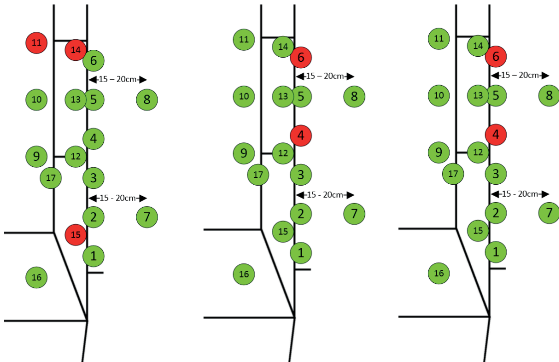
Figure 117: Setup 2 with fixed alarm boundaries and 2dB, 1GHz for: no false alarms (-15 cm), no misses (29 cm), min. wrong decisions (29 cm)
