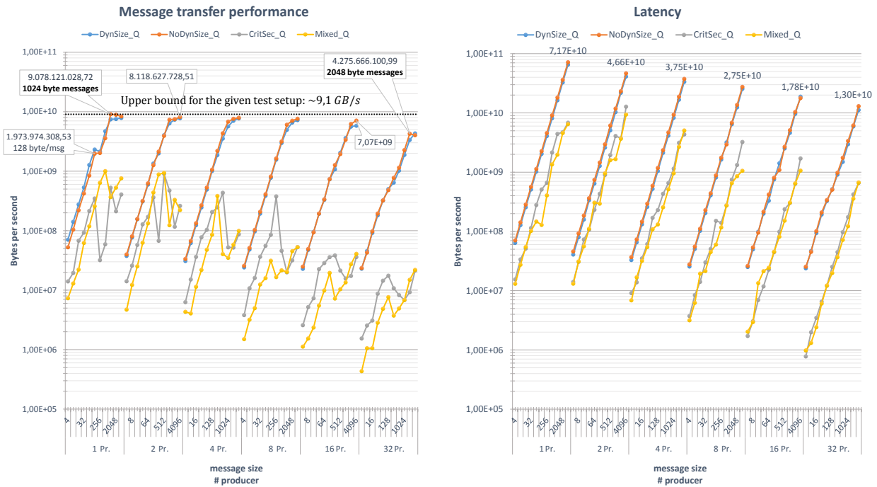
Figure 6.8: Throughput depending on the producers' message size (logarithmic scale). The test setup is equal to the setup in figure 6.6. The results in the left diagram represent the average throughput of 5 test runs, where 17 million messages with a variable payload were sent per test. The diagram on the right hand side illustrates the results without payload. Both diagrams use a logarithmic scale on the y-axis. The message size (the payload) and the number of producers are systematically modified. For all tests the standard deviation from the mean is negligibly small (data not shown).
