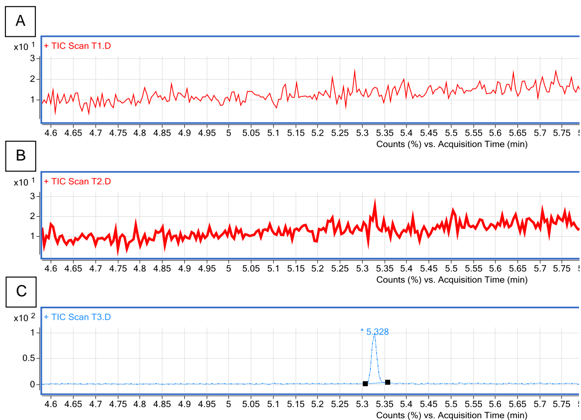
Figure 26: GCMS peak of tested samples after thermic treatment. A: Sample 1; B: Sample 2; C: Samples 3
