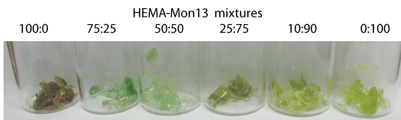
Figure 9. Extraction and swelling test of ATRA-polymers based on HEMA-Mon13 mixtures.
