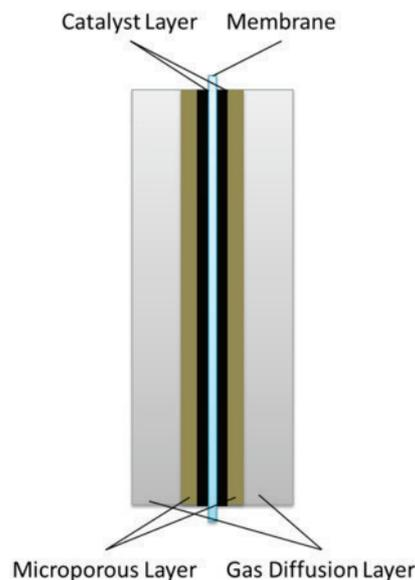
**Figure 4:** Scheme of a membrane electrode assembly.
