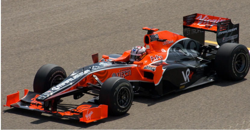
Figure 1.2: Virgin Racing VR-01, the first and only Formula One car designed exclusively via CFD [157]
