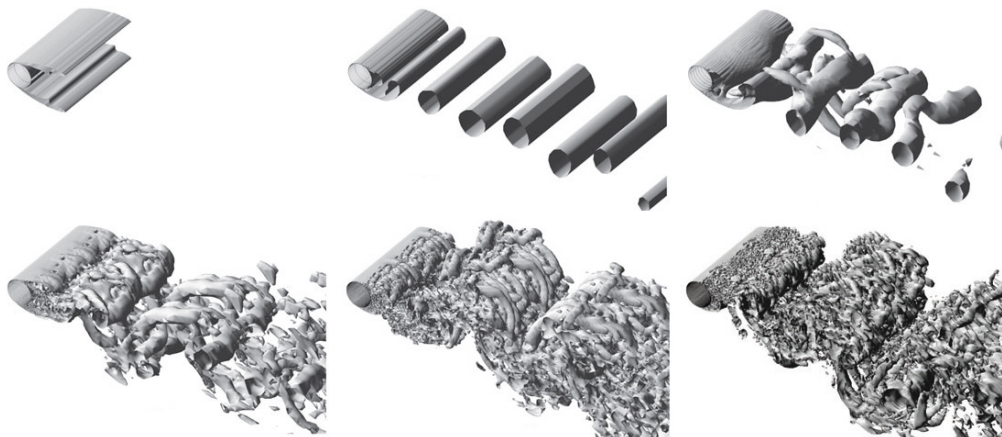
Figure 3.16: Top left to bottom right: RANS, 2d URANS, 3d URANS and DES with three different mesh resolutions [135, 146]
