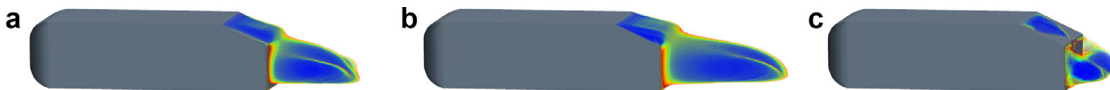
Figure 6.3: Visualisation of the separated flow for the Ahmed body, using the (a) SST RANS, (b) EBRSM RANS and (c) the SST-IDDES model. [12]
