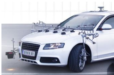
Figure 3.7: Wheel vector system Kistler RV-4 [10]
