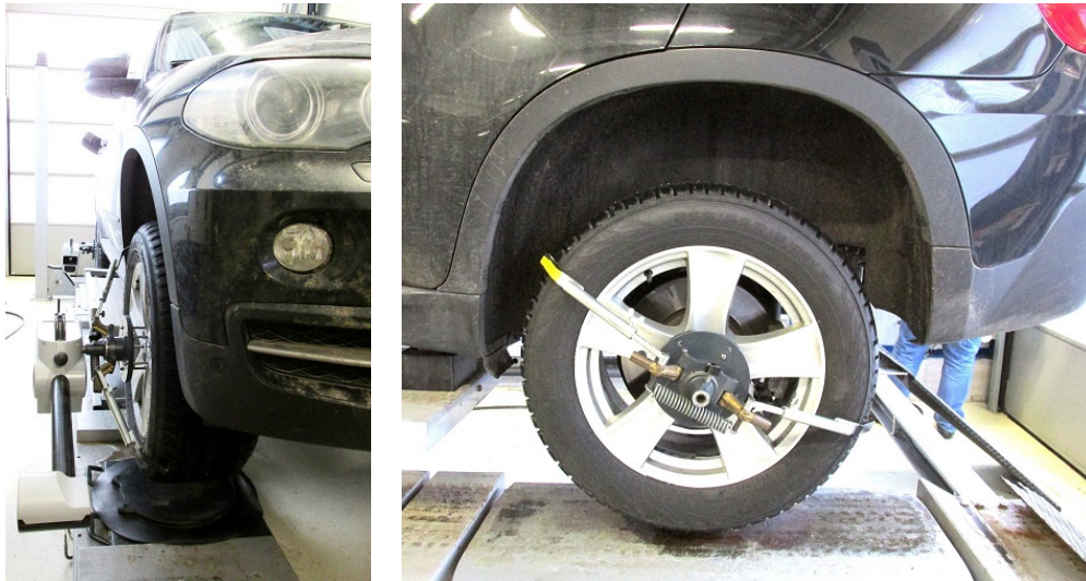
Figure 3.13: Measurement of toe and camber angle of rear suspension at TKP, Eschen
