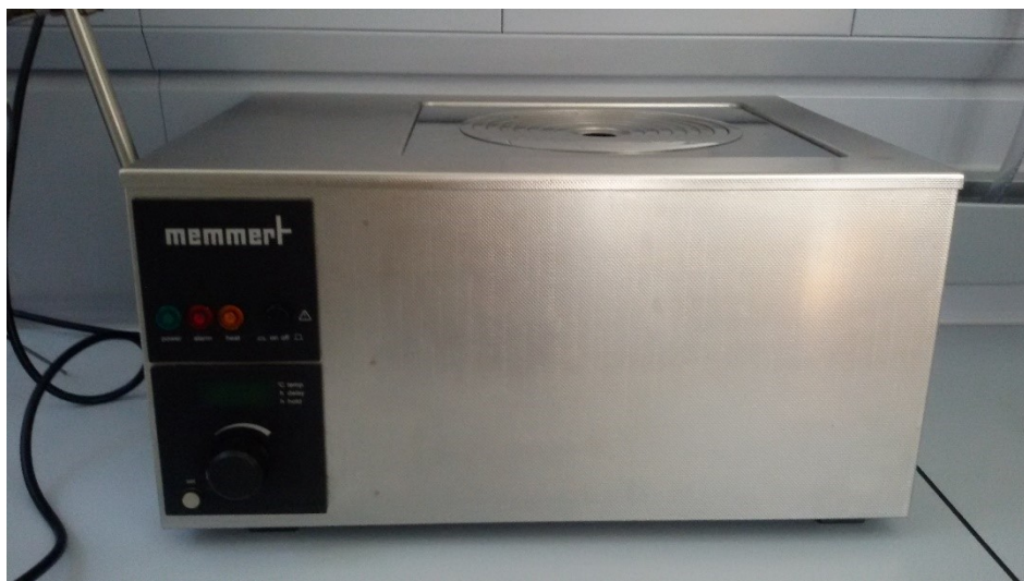
Figure 23: Water bath, Memmert WB7
