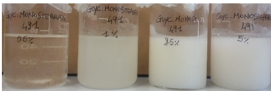
Figure 18: Solution of MCT with IMWITOR 491 CHG.607 395 E (MP 76.2°C) Sasol Germany GmbH
