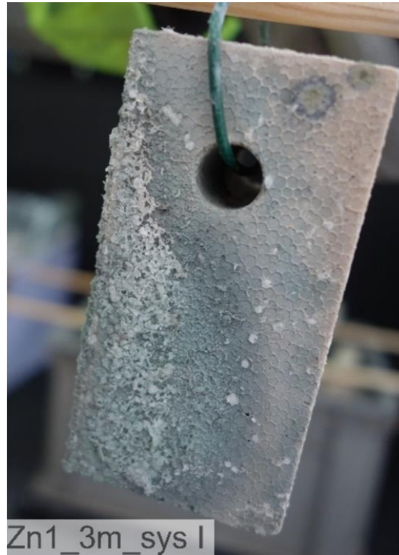
Figure 18: Severe deterioration of the sample GP_Zn1 after 3 months in system I. The mortar contains initially arcanite ( K_2SO_4 ), which was leached out and precipitated on the surface as white-greenish efflorescence. This observation confirms, that sulfates in geopolymer cement mix design have the disadvantage to form soluble sulfates.
