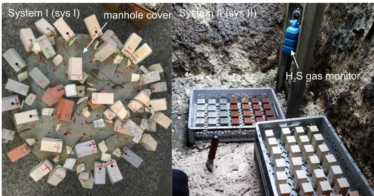
Figure 4: Sample preparation and placing in both systems. In system I, all samples are wire-fixed on the metal inlay beneath the manhole cover. The samples in system II are placed in perforated boxes on an elevated platform. Note the heavily corroded concrete walls of this sewer system. The mushy material on the bottom illustrates the severe deterioration.
