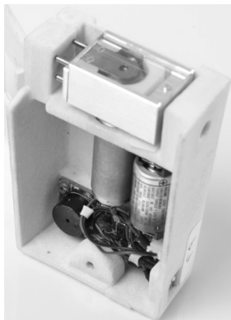
Figure 2-11: First version of a 6-channel microperfusion pump for the operation of 3 OFM probes in push-pull mode (size 10 x 5 cm)
