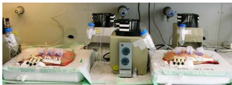
Figure 2-19: Ex vivo set-up comparing OFM and MD in two human skin explants. One explant was treated with fentanyl, the other with benzoic acid.
