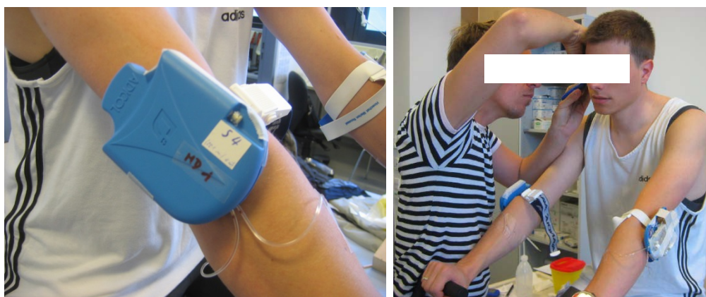
Figure 2-21: Lactate monitoring in forearm skin using a wearable pump and a dermal OFM probe
