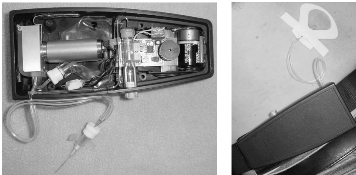
Figure 2-6: First version of the wearable 2-channel OFM pump for the sampling from a subcutaneous OFM probe (Year 2002)
