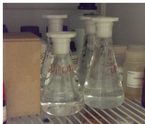
Figure 29: Bubblefree cooled storage using Erlenmeyer flasks and polymere plugs
