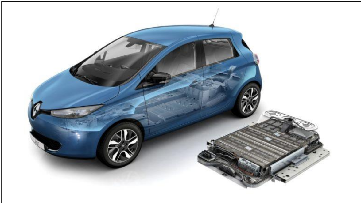
Figure 10.2 Renault ZOE battery pack 240
