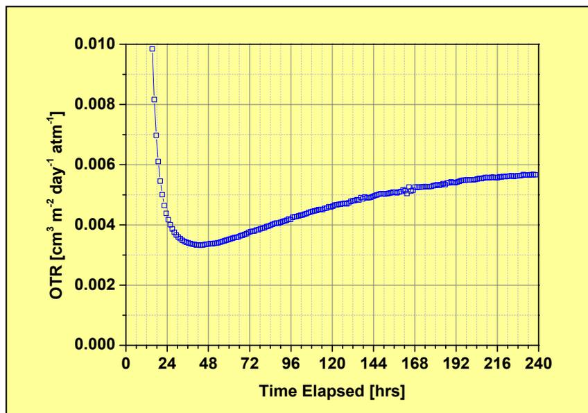
Fig. 5-25: The course of OTR results obtained for a complex multi-layer barrier membrane. During the first 24 hours, oxygen dissolved in superficial layers of the membrane is desorbing and dominates the amount accumulating in the receiving cavity. The establishment of steady-state permeation requires about 10 days with this sample. In the transition between desorption of dissolved oxygen and actual permeation, intermediately constant results may be mistaken for the completion of the measurement.
