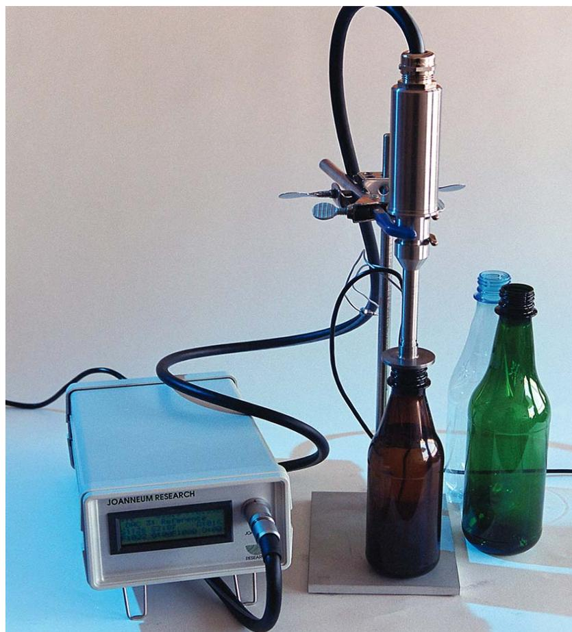
**Fig. 4-3:** An opto-electronic setup as it was used in the development of the OTR measuring instrument. The setup comprises the “vector board” (digital readout electronics, grey enclosure left) and the “probe” (steel cylinder on top of a beer bottle, mid-right). The image illustrates the setup used for the measurement of oxygen in the headspace of beer bottles [81].
