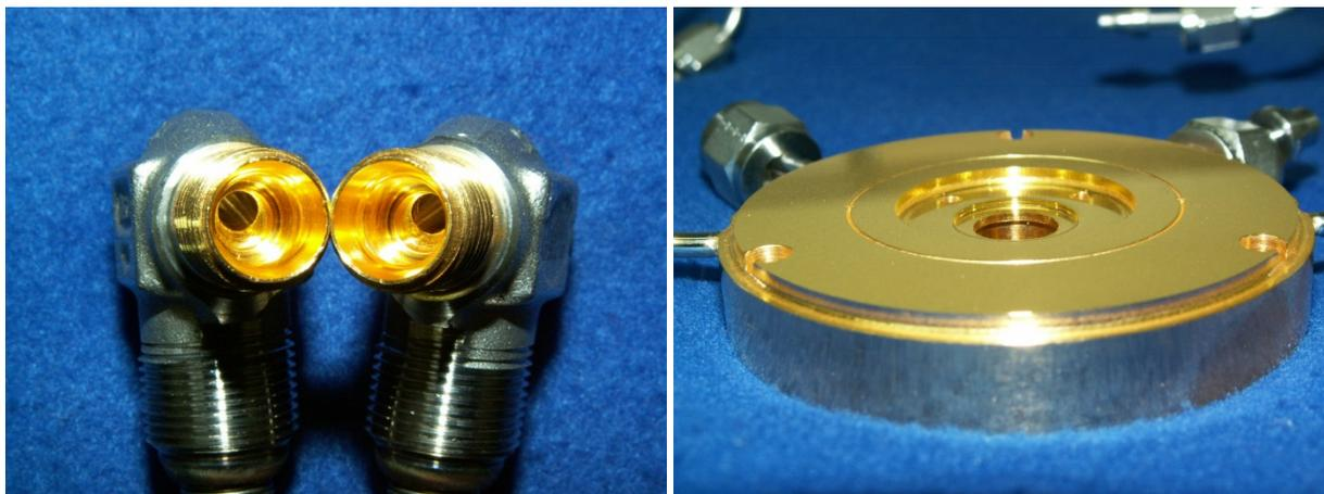
**Fig. 5-15: The functional surfaces of the OTR measuring cell were gold-coated by means of “Pulsed Laser Deposition”.**
