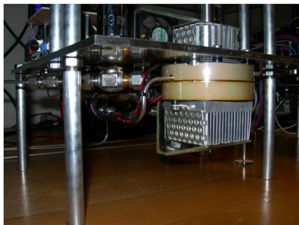
**Fig. 5-16: The Completed Assembly of the OTR Measuring Device. In the Background of the Left-hand Image, the Device Used for Routine Measurements is also seen.**
