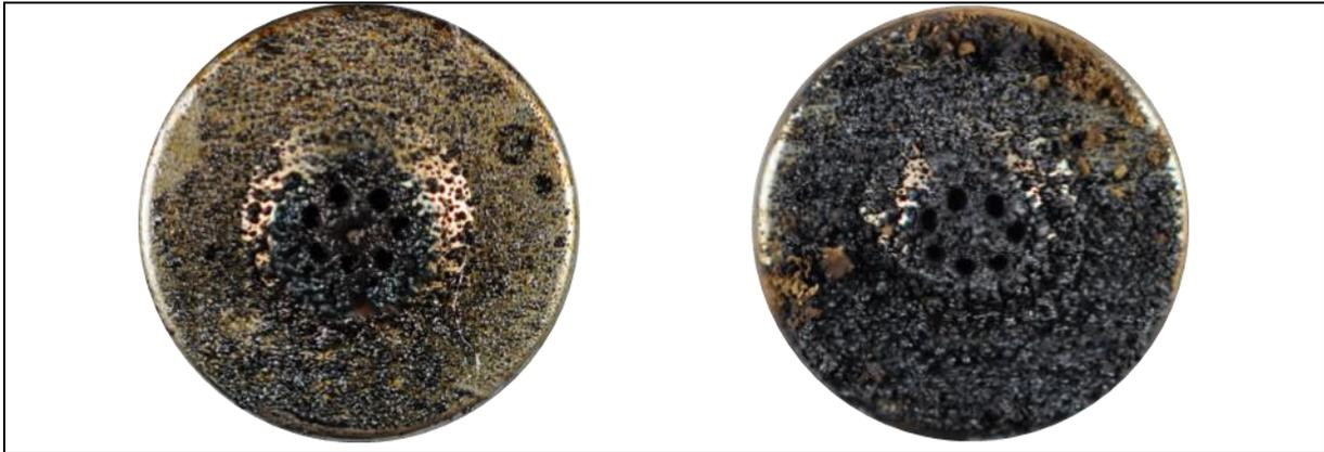
Figure 86: Coked injectors from China 92 deposit test runs from cylinder 1 (left) and 2 (right).
