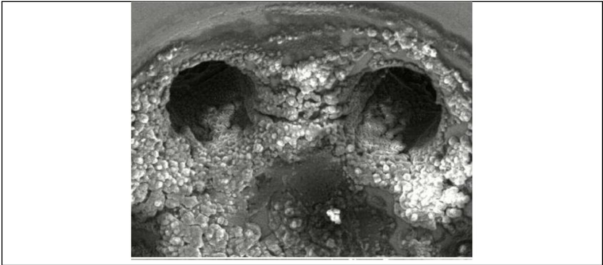
Figure 13: Deposits inside the injector nozzle (internal deposits) [39]
