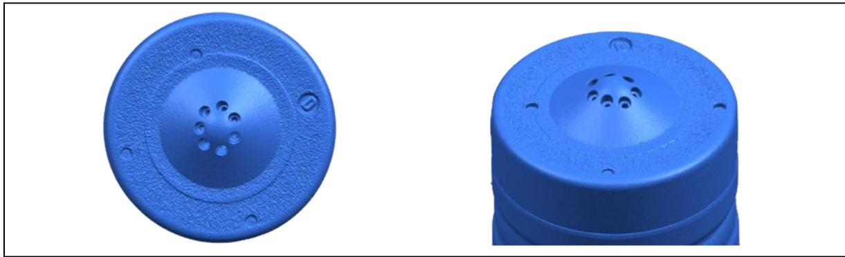
Figure 44: Injector STL File converted from X-Ray
