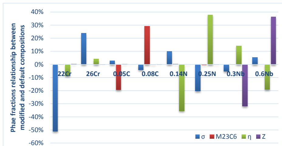
Figure 37: Influence of Cr, C, N, Nb on equilibrium phase fractions at 650°C.
