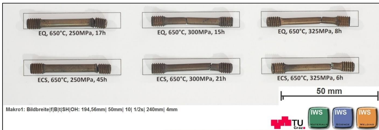
Figure 47: Creep samples ruptured at 650°C.
