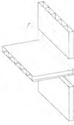
Figure 2-39: Platform building method (steel-frame construction) 95
