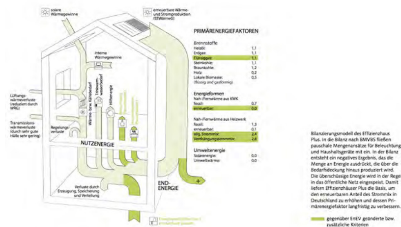
Figure 2-14: Balance Model for the Efficiency-house Plus. 73
