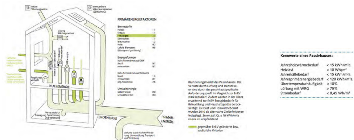
Figure 2-12: Balance model for a Passive house with main parameters. 71
