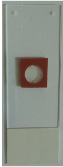
Figure 2.7: One secure seal applied to a superfrost slide. The secure seal chambers are available with different reaction volume capacities starting from 35 \mu\text{l} up to 620 \mu\text{l} . For our approach we use 50 \mu\text{l} chambers. The chambers can be filled with a pipette through one of two small holes. During pipetting, bubble formation should be avoided.
