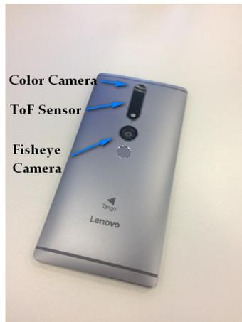
Figure 1.1: Picture of the backside of the Lenovo Phab 2 Pro. Sensors seen include a color camera, a ToF sensor, and a monochromatic fish eye camera.
