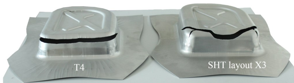
Figure 71 left: crack formation T4 state; right: crack formation SHT layout X3
