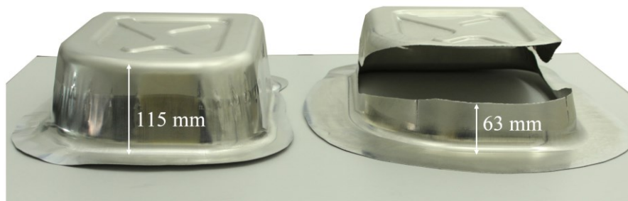
Figure 78 left: formed part due to optimal SHT process parameter; right: formed part without SHT
