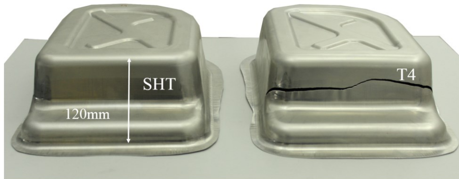
Figure 80 Multi-stage forming process: left: formed part through SHT; right: formed part without SHT in the process
