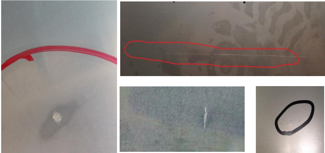
Figure 24: Collection of detected scratches on the raw material
