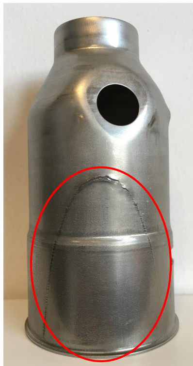
Figure 1: u-curve fault pattern
