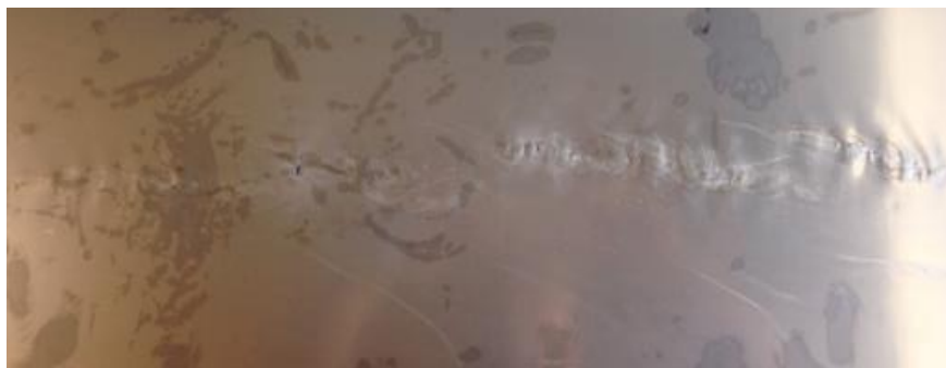
Figure 25: Deformation on the coil
