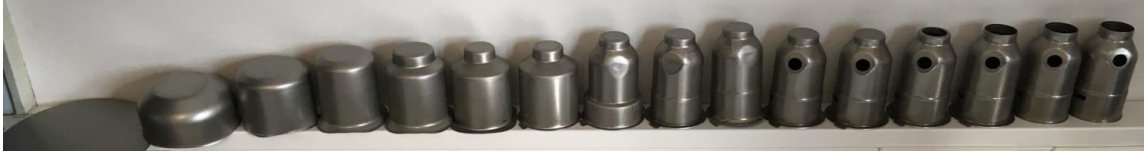
Figure 23: 15 steps of drawing process
