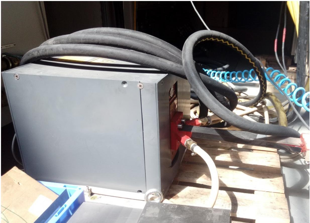
**Figure 3-45:** Induction heating system of the TU Graz
