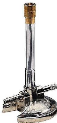
Figure 4.6: primary=gas (methane), suction=gas (air): Bunsen burner [23]
