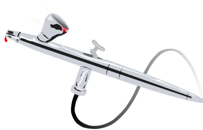
Figure 4.7: primary=gas (air), suction= liquid (paint): Airbrush [25]
