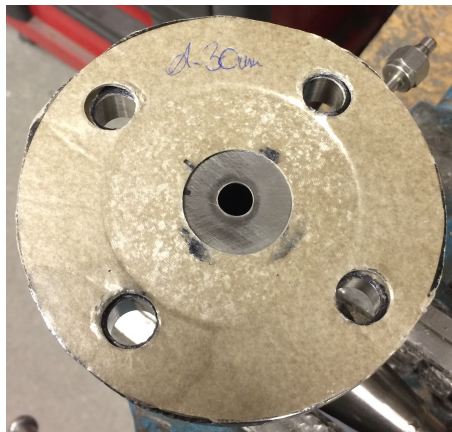
Figure 5.7: Orifice Suction with flange and high-temperature sealing
