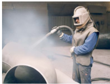
Figure 4.8: primary=gas (air), suction=solid (sand): Sandblasting [27]
