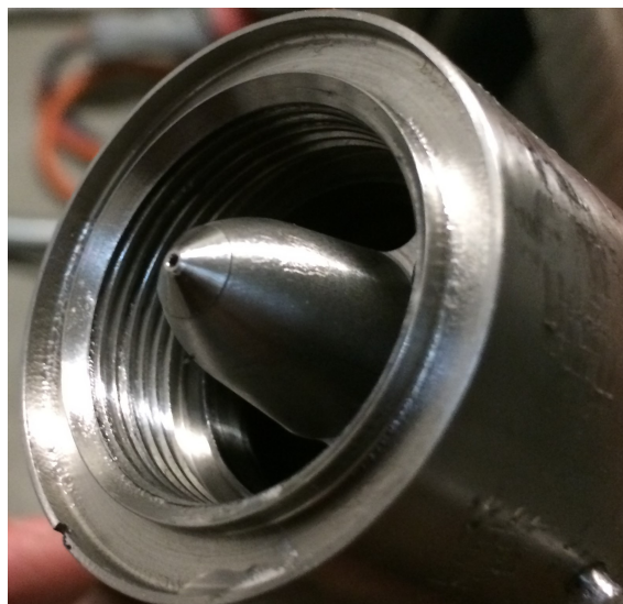
Figure 5.9: Nozzle-holder without step: POS 3 (Ejector test system design A)
