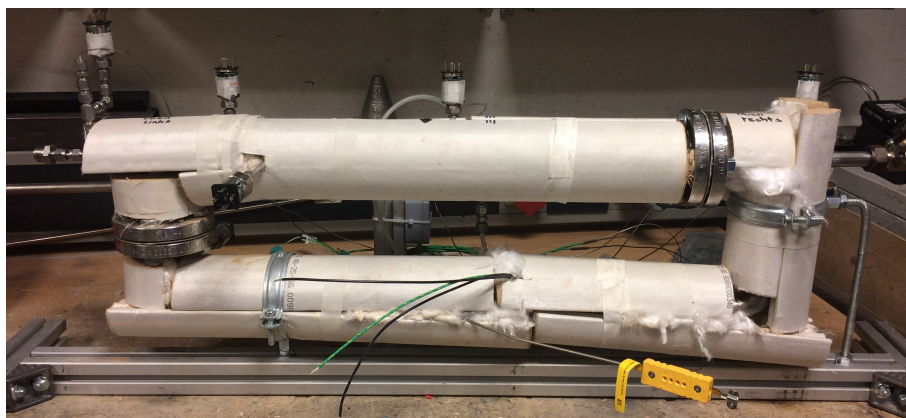
Figure 5.3: Laboratory preparation of test rig for the closed case (Ejector test system design A)
