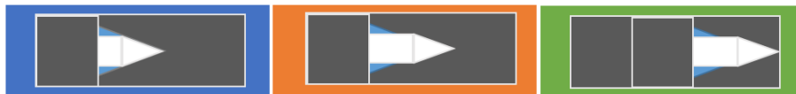
Figure 6.3: Position variation of the nozzle and the nozzle holder (POS 3 , POS 2 , POS 1 ) from left to right
