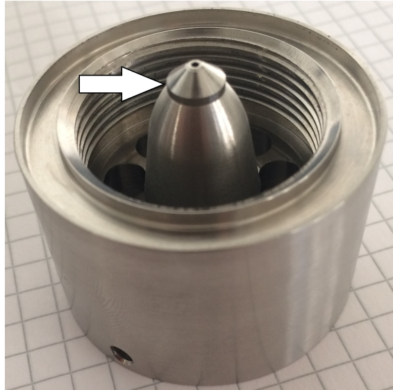
Figure 5.8: Nozzle-holder with step: POS 1 and POS 2 (Ejector test system design A)
