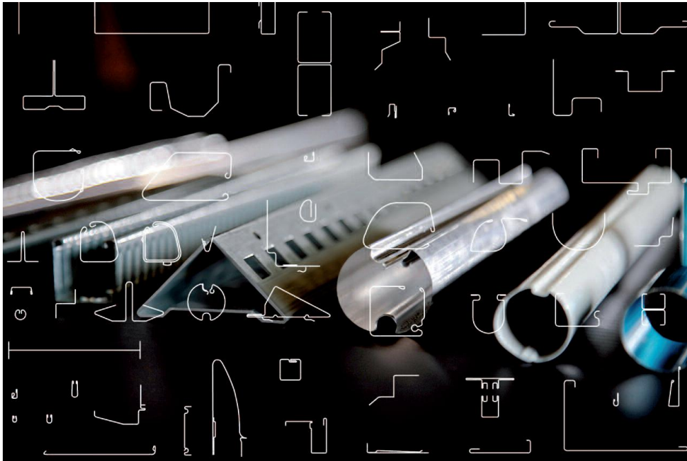
Figure 1: Roll formed profiles for different industries [Wag11]
