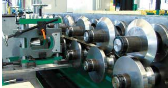
Figure 12: Cantilevered mill type [Sch13]
