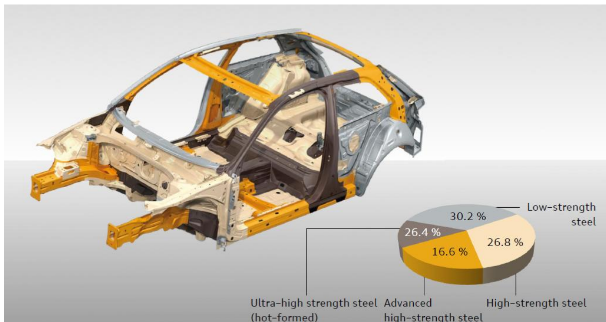
Figure 74: Car body material mix of the new Audi A3 [Pii12]
