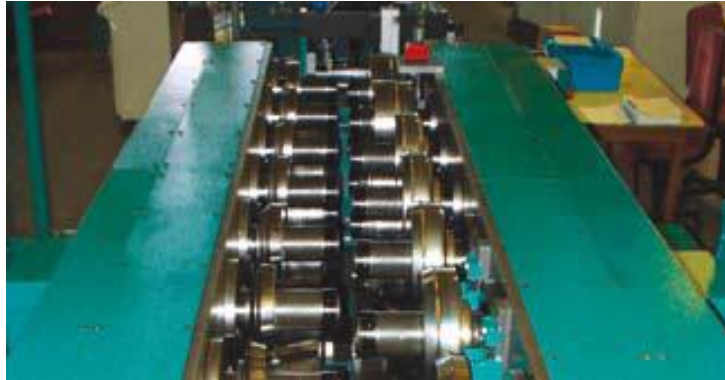
Figure 18: Duplex mill type [Sch13]
