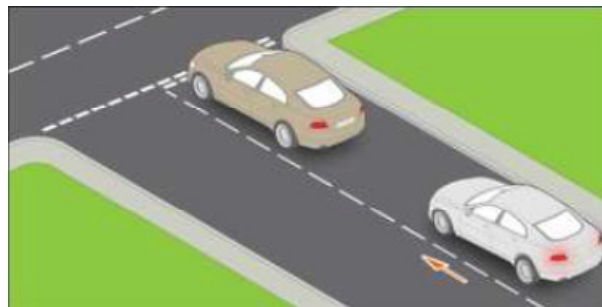
Figure 26 Approaching a stopped vehicle at test speeds from 10 to 60km/h [33]
