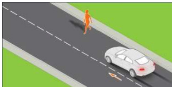
Figure 30 Unobscured pedestrian walks out from nearside [33]
