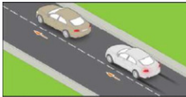
Figure 28 Approaching a moving target at 20km/h [33]
