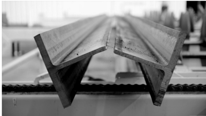
Figure 18 : A bisected I beam into two T-sections [6]
