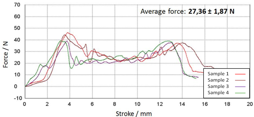
Figure 86: Results peel test: Force-stroke-diagram of RU302507V01 (5) (four samples) and calculated average force for this surface modification.
