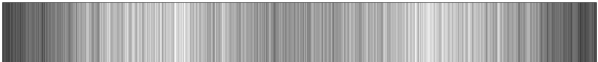
Figure 25: Dark field image of a 4096 \times 1 pixel array detector with two particles within measuring volume. Each stripe indicates a single pixel element. Due to the fact, that no optic was used to focus the scattered light, a counting analysis is almost impossible. Therefore an imaging optic is necessary. List of parameters: see appendix (section 8).
