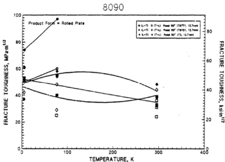
Figure 5-5 Fracture toughness over temperature for alloy 8090 [28]
