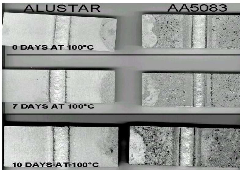
Figure 5-3 Surface of sensitized samples after the ASSET Test [25]
