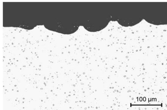
**Figure 2-20 Example of flat pitting corrosion in AlMg alloy attacked by an alkaline agent [20]**
