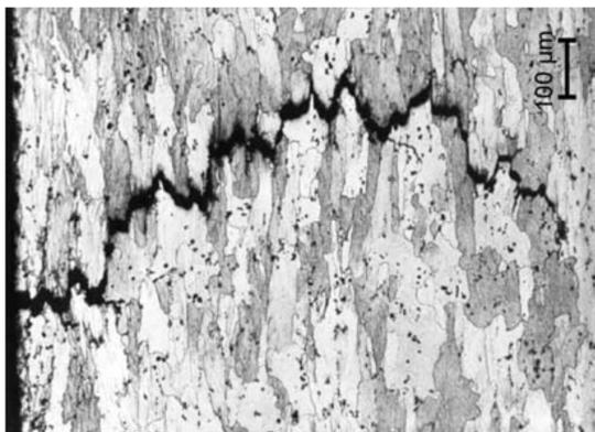
Figure 2-26 Intergranular corrosion in tension in Al-Cu alloy [20]
