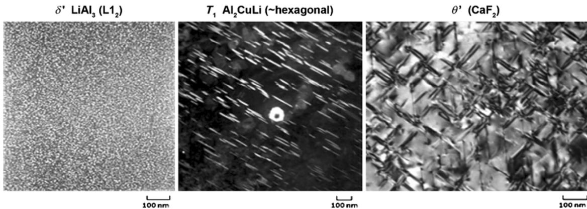
Figure 2-5 Strengthening precipitates in 3rd generation Al-Li alloys [11]
