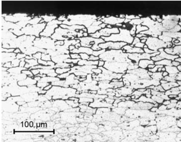
Figure 2-23 Example of intercrystalline corrosion in Al-Mg alloy [20]
