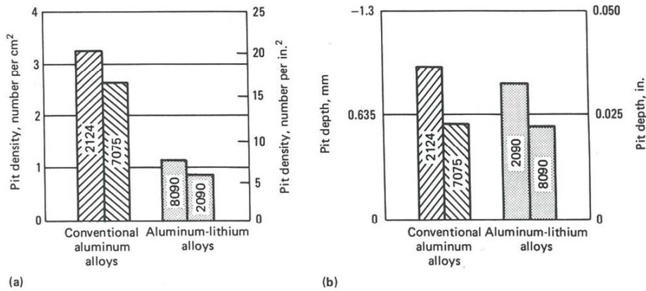
**Figure 2-19 Pitting characteristics of selected aluminum and aluminum-lithium alloys exposed to an SO<sub>2</sub> salt fog for 32 days. [2]**
