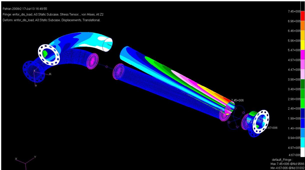
**Figure 6-3 FEM Analysis of Aluminum Feed Line Enforced Displacement**
