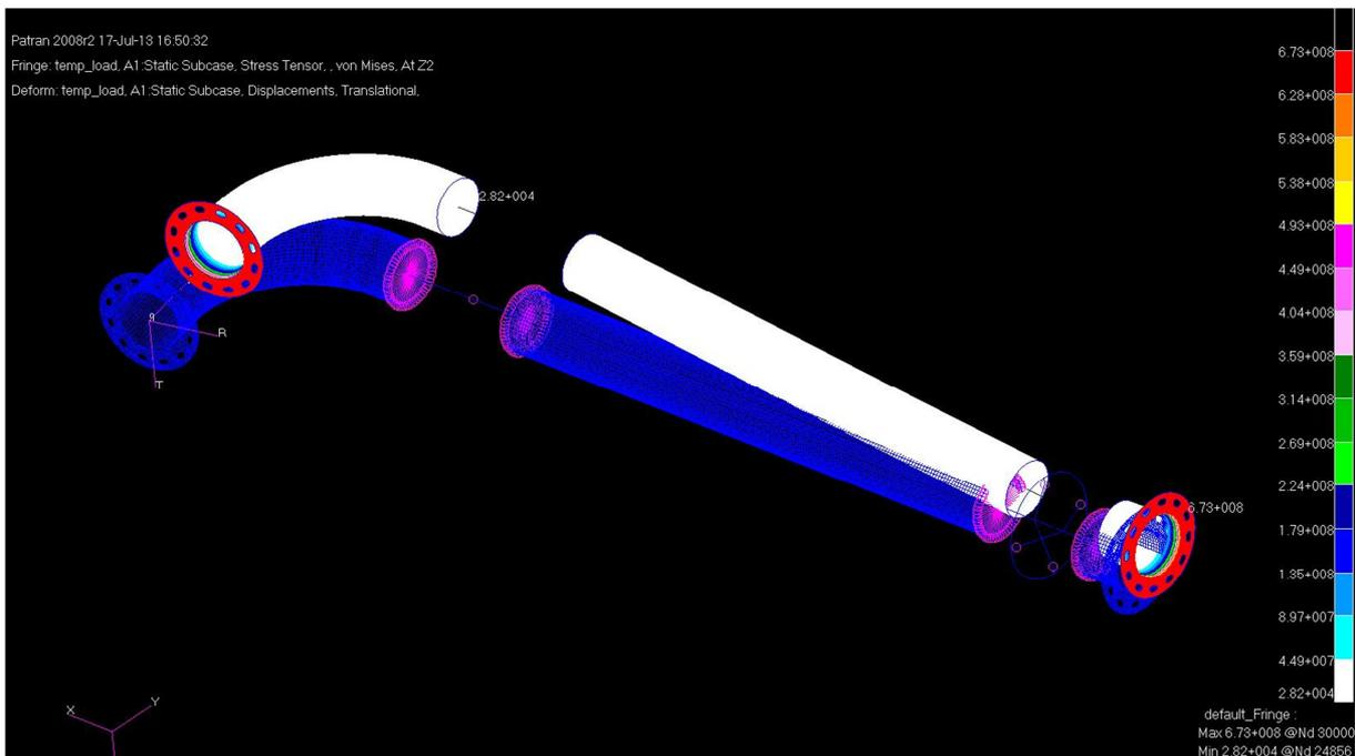
**Figure 6-4 FEM Analysis of Aluminum Feed Line Thermal Expansion**
