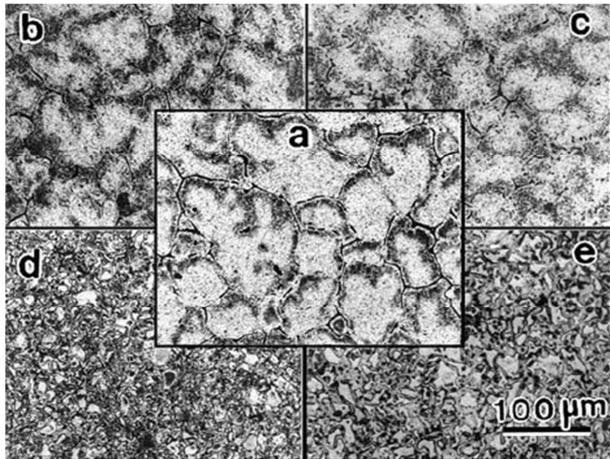
**Figure 2-11** Grain Size of as cast Al-Li alloys haing 0.1%Zr and 0%Sc (a), 0.11%Sc (b), 0.22%Sc (c), 0.43%Sc(d) and 0.84%Sc(e) [15]
