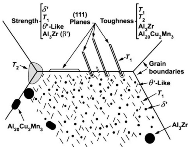
Figure 2-4 Schematic precipitate microstructure in Al-Li 2099 and 2199 alloys [11]
