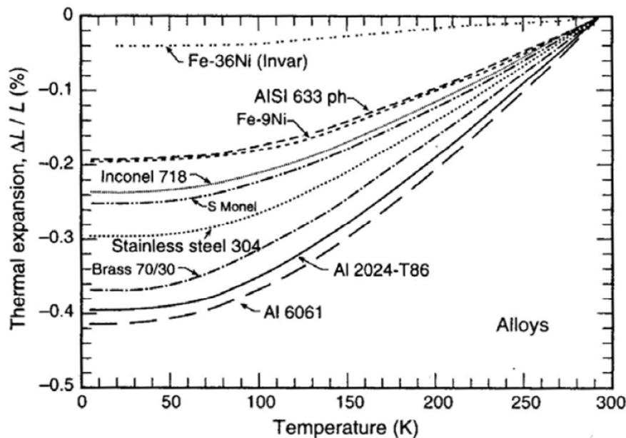
Figure 2-17 Thermal expansion of different materials [19]
