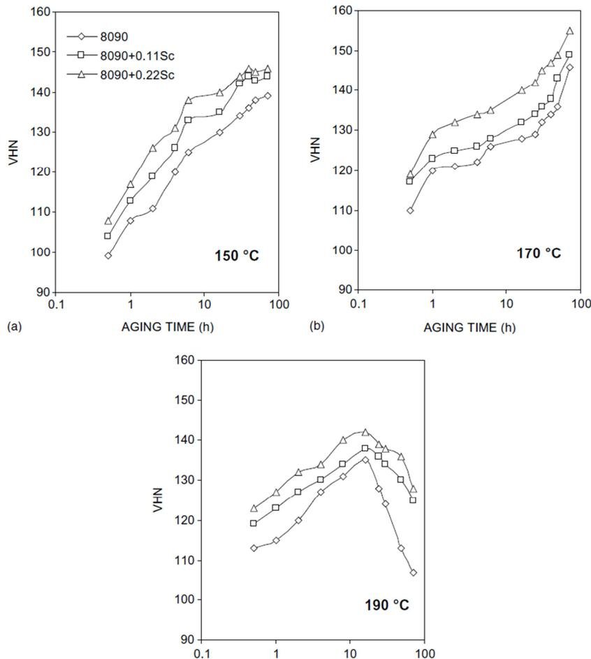
**Figure 2-14 Hardening curves for the alloys 8090, 8090+0.11%Sc and 8090+0.22%Sc aged at different temperatures [15]**
