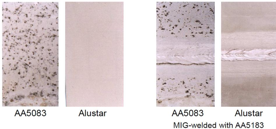
Figure 5-2 ASSET Corrosion Test Results before and after Welding [25]
