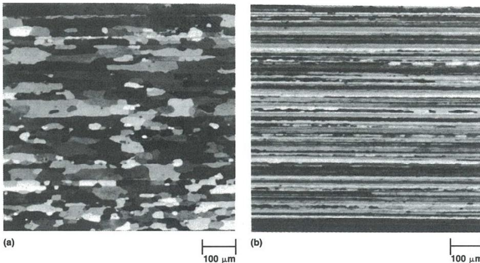
**Figure 5-4 Recrystallized and unrecrystallized grain structure of AA8090 sheet**
