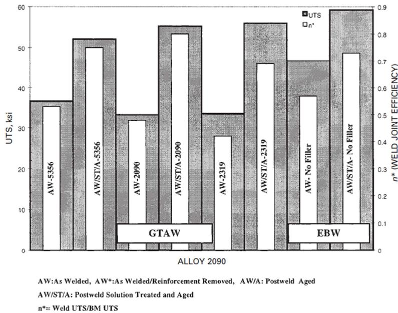
Figure 2-15 Weld joint efficiency for alloy 2090 using various processes and filler metals [12]
