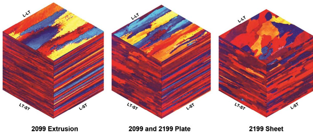
Figure 2-7 Optical micrographs showing an extruded product with thin, elongated unrecrystallized grains; a plate product with elongated unrecrystallized grains; and a sheet product with recrystallized grains [11]
