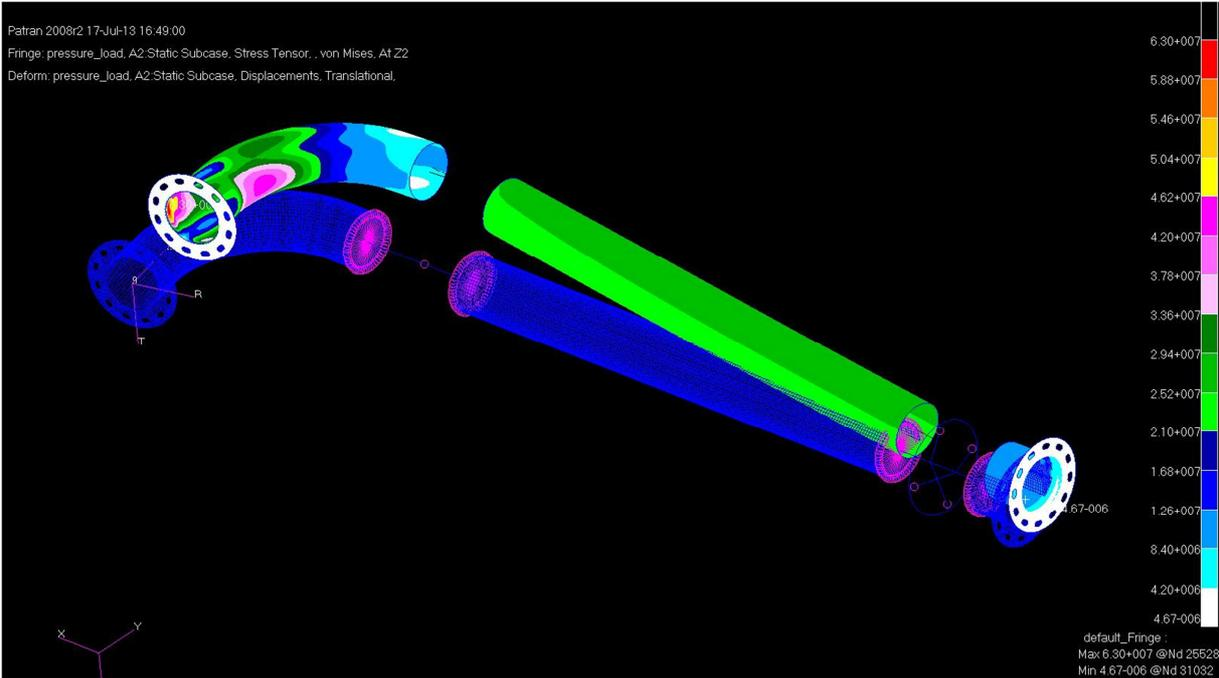
Figure 6-2 FEM analysis of Aluminum Feed Line Pressure Load
