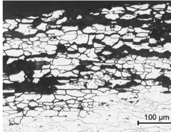
Figure 2-22 Example of intergranular corrosion in an Al-Mg alloy due to insufficient quenching rate at tempering [20]
