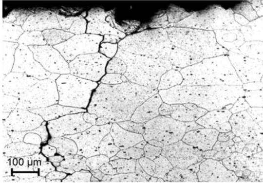
Figure 2-25 SCC in alloy 7020 showing intergranular fracture in recrystallized microstructure [20]
