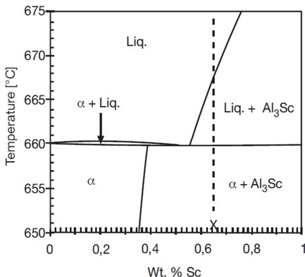
Figure 2-8 Sketch of the Al-rich side of the Al-Sc phase diagram. The symbol X indicates an arbitrary hypereutectic composition [14]
