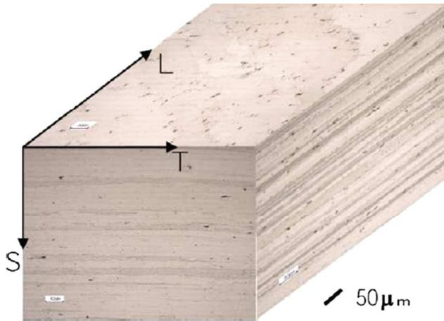
Figure X Pseudo 3D Image of the grain structure [16]
