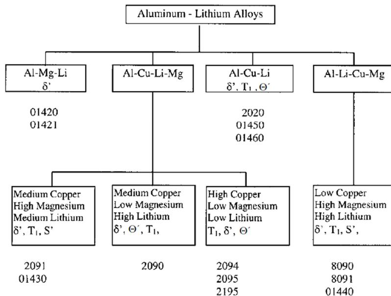
Figure 2-3 Classification of Al-Li Alloys [12]
