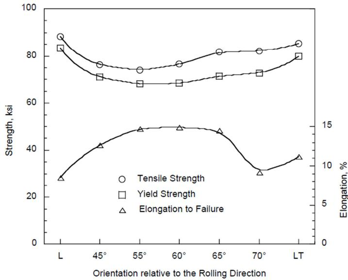
Figure 5-9 Strength and Elongation depending from rolling direction for alloy 2195 [30]
