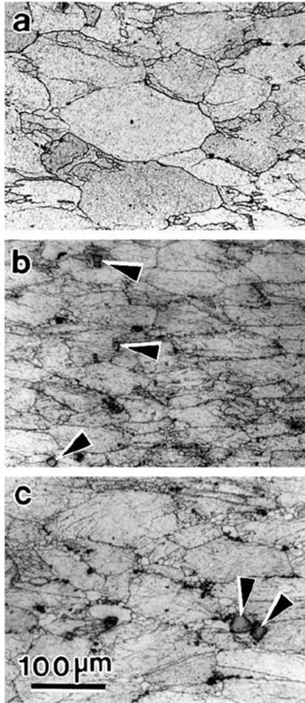
**Figure 2-12** Optical micrographs of forged and T8 heat treated alloy 8090 (a), 8090+0.11%Sc (b) and 8090+0.22%Sc (c) [15]
