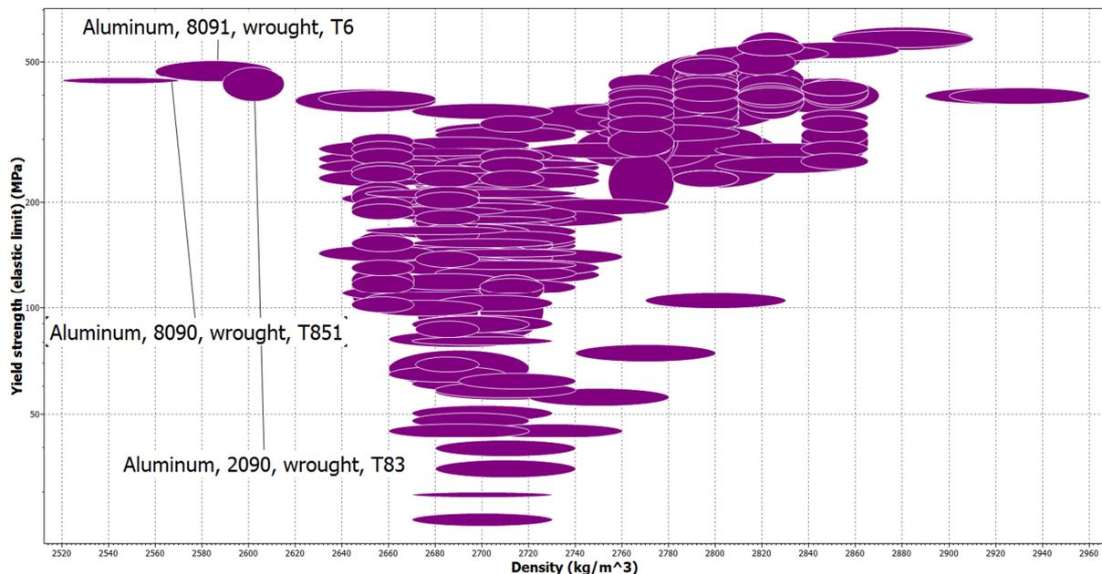
Figure 4-1 CES Plot of Aluminum Alloys
