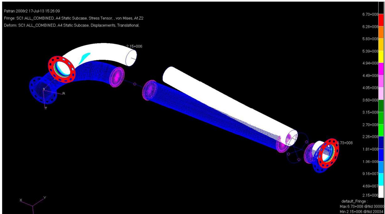
**Figure 6-5 FEM Analysis of Aluminum Feed Line Combined Load**
