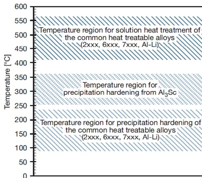
Figure 2-10 Typical temperature regions for solution heat treatment and precipitation hardening of the common heat treatable alloys, and for precipitation hardening from Al<sub>3</sub>Sc [14]
