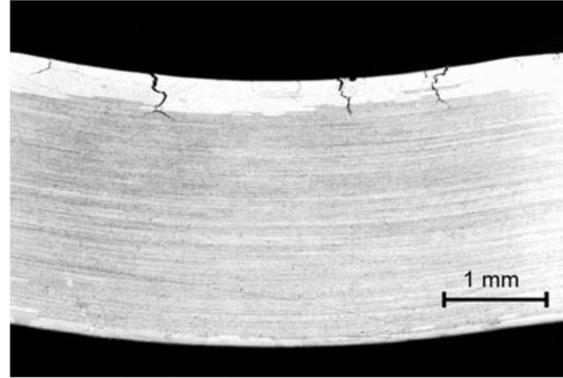
Figure 2-24 SCC in Al-Zn alloy showing intergranular fracture in recrystallized coarse grain zone [20]
