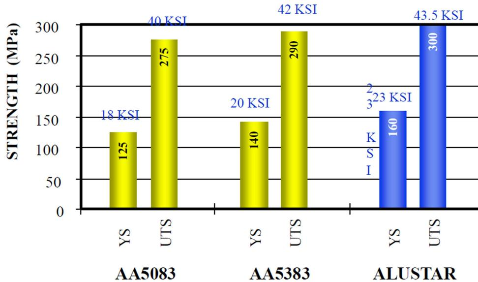
Figure 5-1 After weld strength of MIG welded plate [25]
