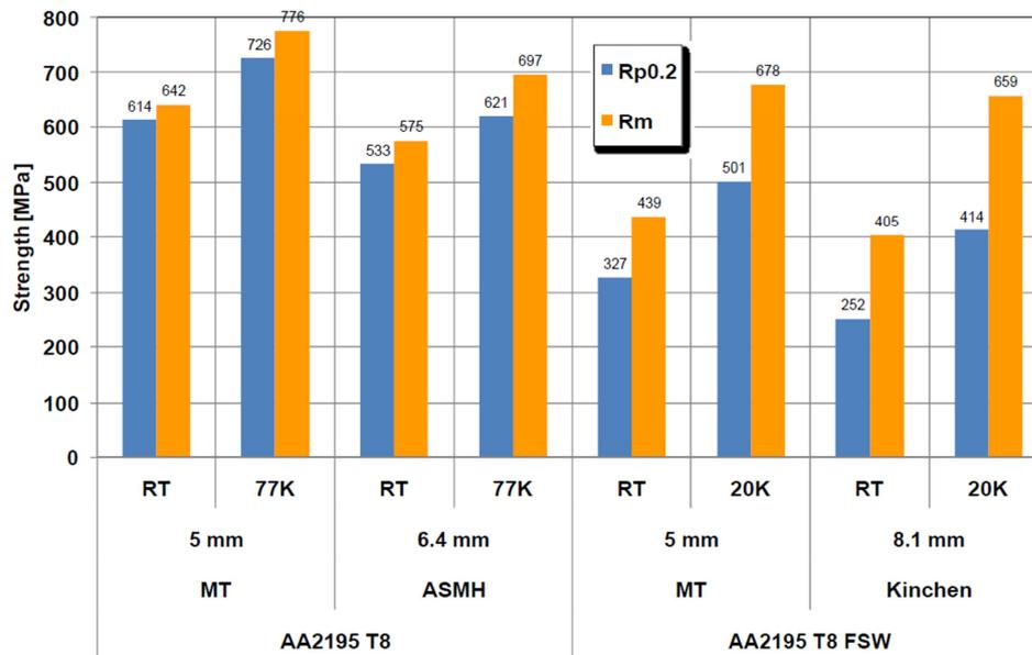
Figure 5-10 Strength of 2195 base material and FSW weldments
