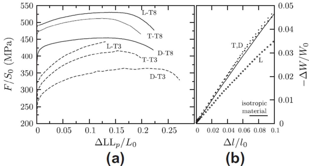
**Figure 5-11 Tensile tests of alloy 2198 in different directions**
