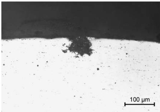
**Figure 2-21 Example of deep pitting corrosion in AlMg alloy attacked by an acidic agent [20]**
