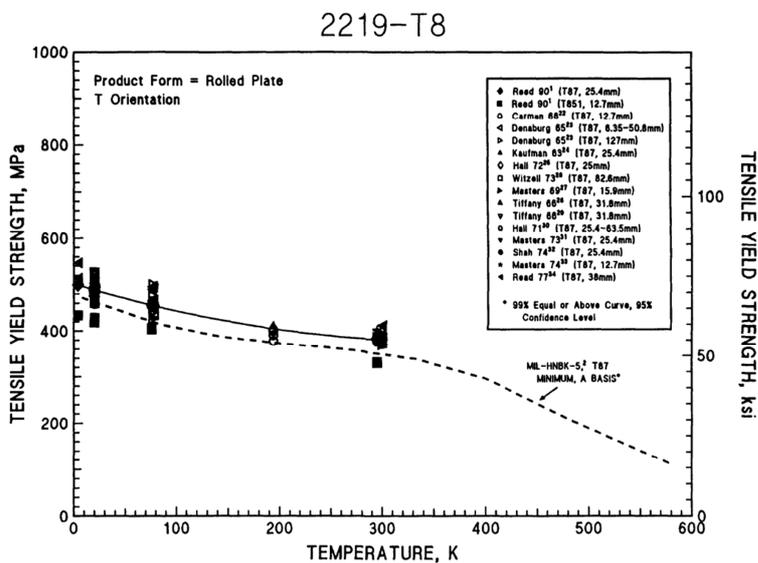
Figure 5-7 Yield Strength of Alloy 2219 T8- T Orientation [29]
