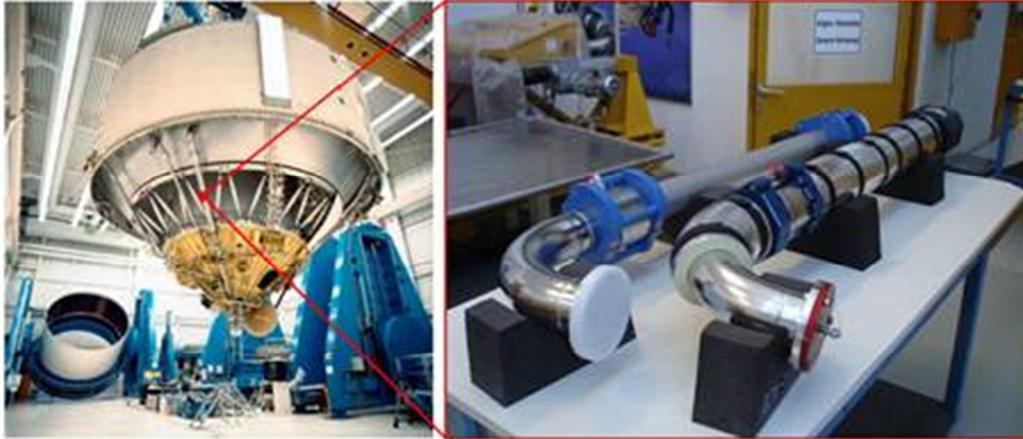
**Figure 1-1 Fuel line of Ariane 5 upper stage engine, picture by Magna Steyr**
