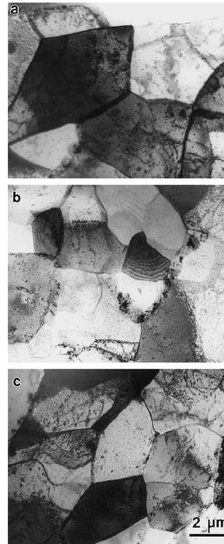
**Figure 2-13** Transmission electron micrographs of alloy 8090 (a), 8090+0.11%Sc (b) and 8090+0.22%Sc (c) in T8 condition [15]
