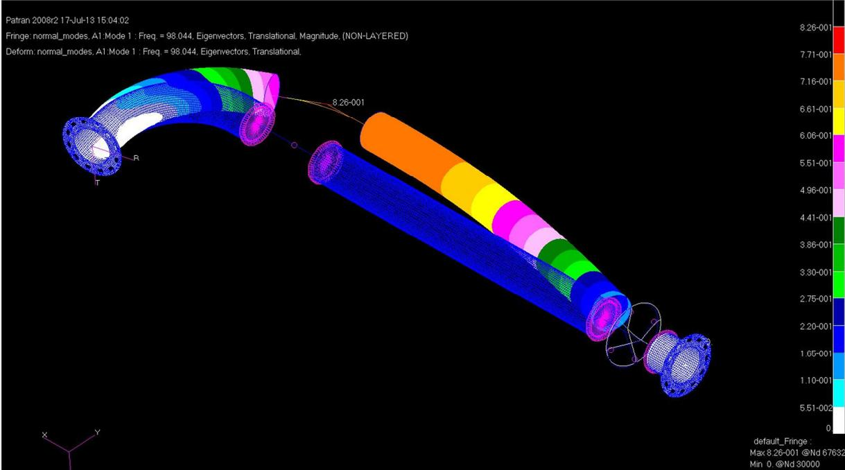
Figure 6-1 FEM Analysis of Aluminum Feed Line Eigenfrequency
