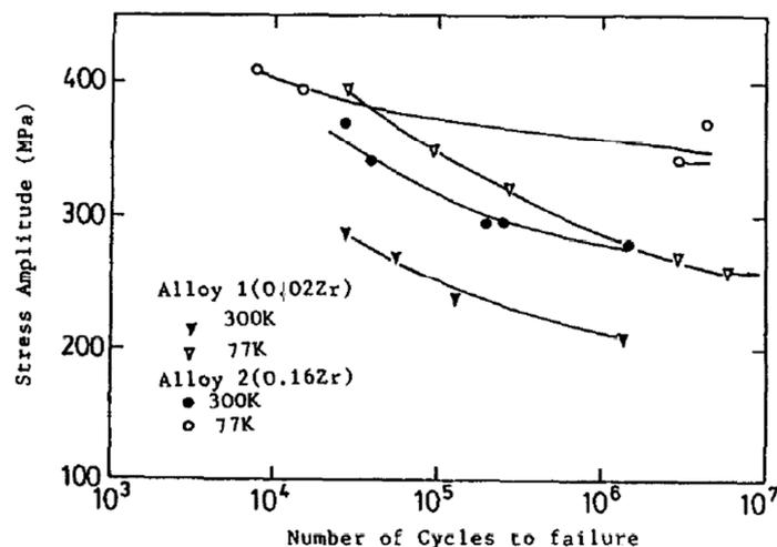
Figure 2-2 Fatigue curves of Al-Li-Cu-Mg-Zr alloys fatigued at 300K and at 77K [8]
