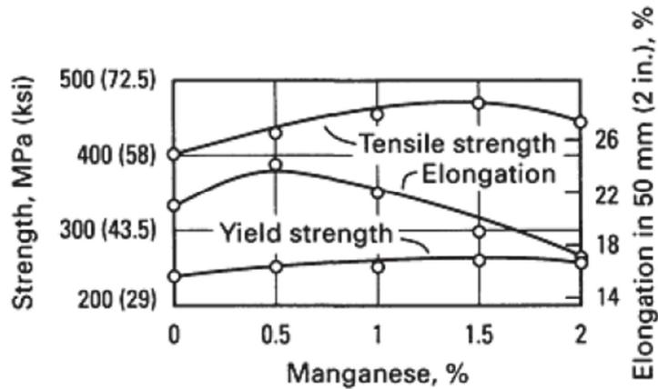
Figure 2-1 Effect of Manganese addition on Strength and Elongation [2]
