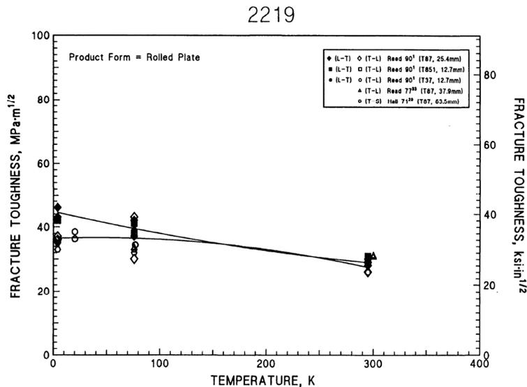
Figure 5-8 Fracture Toughness vs. Temperature of Alloy 2219 [29]
