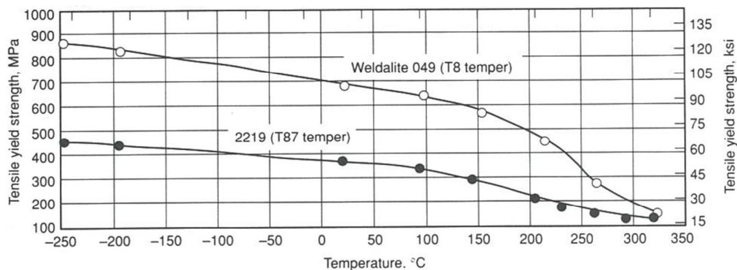
Figure 2-18 Yield strength comparison of an aluminum-lithium candidate alloy for cryogenic tankage applications with a conventional alloy [2]
