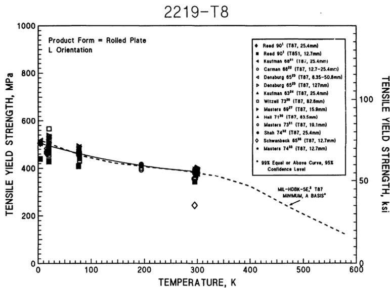
Figure 5-6 Yield Strength of Alloy 2219 T8- L Orientation [29]
