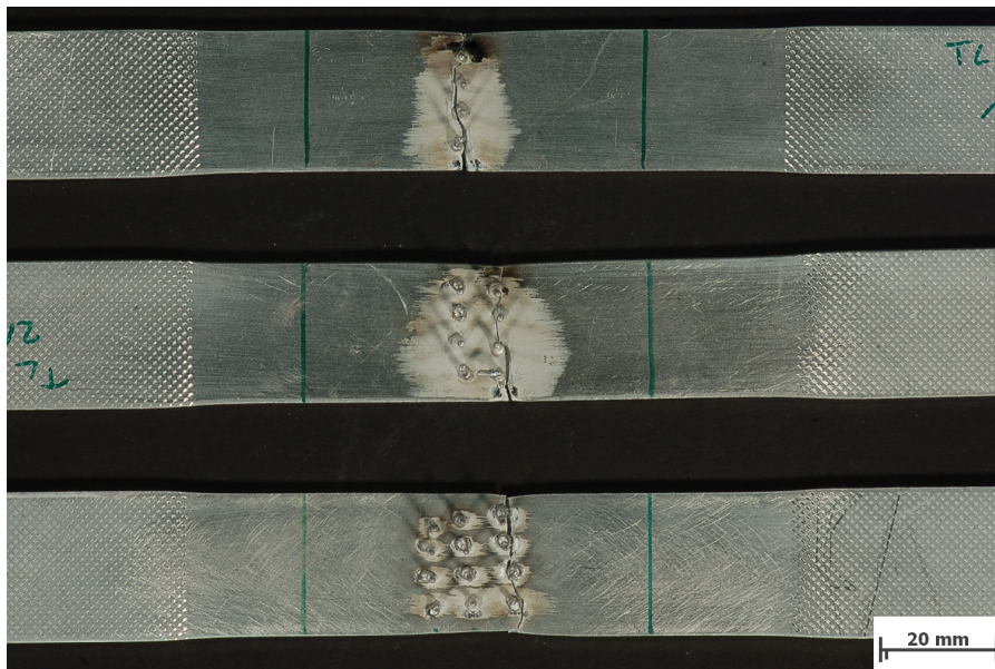
Figure 3.22.: Fracture patterns of AA6xxx alloy samples with classic CMT pins
