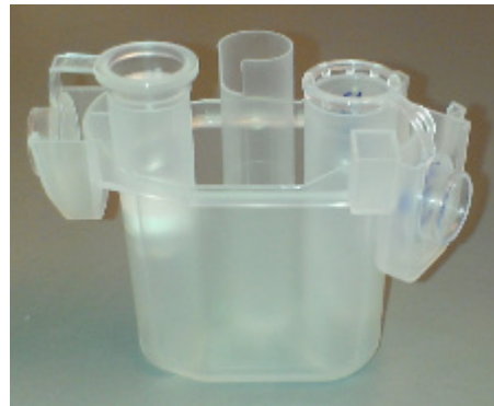
Figure 26: rotor adapter including on the left side the spin column and on the right side the Elution tube
