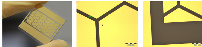
Figure 4.17: Inverted photolithography mask for the fabrication of transparent trenches, with an average line width of 150\text{ }\mu\text{m} .
