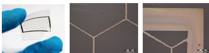
Figure 4.11: Photography of the silver grid printed on PEN foil (left), microscopy images of the printed silver grid on PEN (middle, left).
