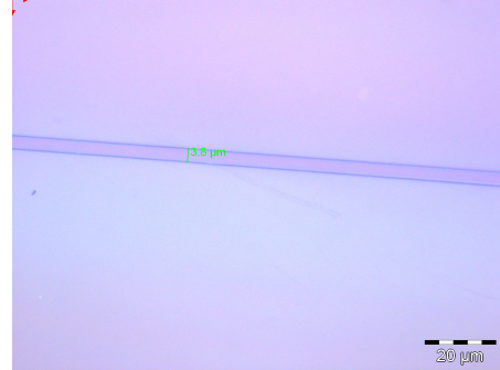
Figure 4.16: Microscope picture of test line with minimal lateral resolution, using 40XT as a photo resist on PET foil, with the standard process parameters.
